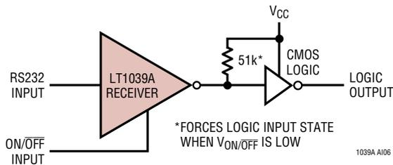
To protect against receiver input overloads in excess of  $\pm 30V$ , a voltage clamp can be placed on the data line and still maintain RS232 compatibility.
