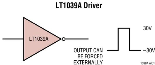
The driver outputs utilize high impedance overvoltage protection, eliminating the flow of fault currents into supplies, as will happen with conventional diode clamp-configurations.
