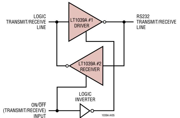
The shutdown mode also drops all supply currents ( $V_{CC}$ ,  $V^+$ ,  $V^-$ ) to zero for power conscious systems.
