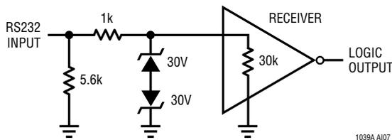
The receiver input impedance of the LT1039A is nominally 30k $\Omega$ . For applications requiring a 5k $\Omega$  input impedance, a 5.6k resistor can be connected from the receiver input to ground.
