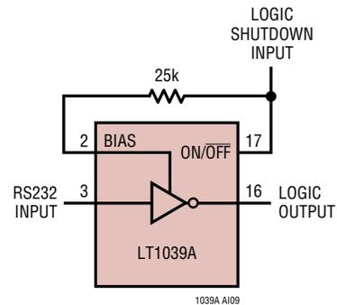
It can also be used to make an RS232 compatible shutdown control line. Driving the BIAS pin low through a resistance of 24k to 30k keeps the receiver active. Do not drive the BIAS pin directly from a logic output without the series resistor. An unused BIAS pin should be left open.
