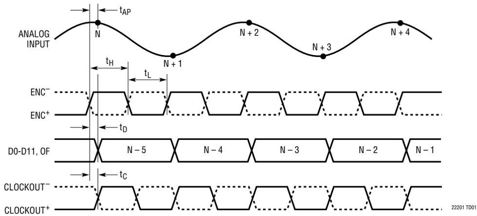
**Full-Rate CMOS Output Mode Timing**
