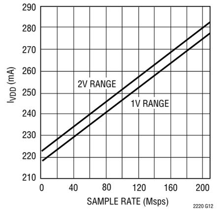
**LTC2220:  $I_{OVPD}$  vs Sample Rate, 5MHz Sine Wave Input, -1dB**
