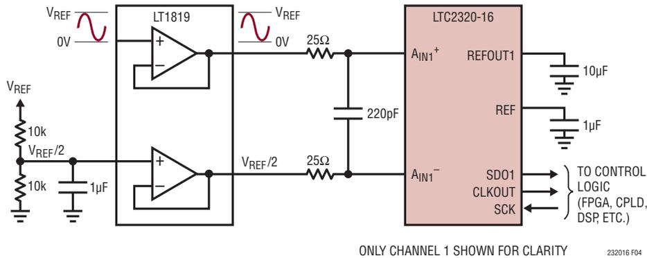
Figure 4. Pseudo-Differential Bipolar Application Circuit
