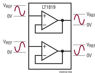
Figure 9. LT1819 Buffering a Fully-Differential Signal Source
