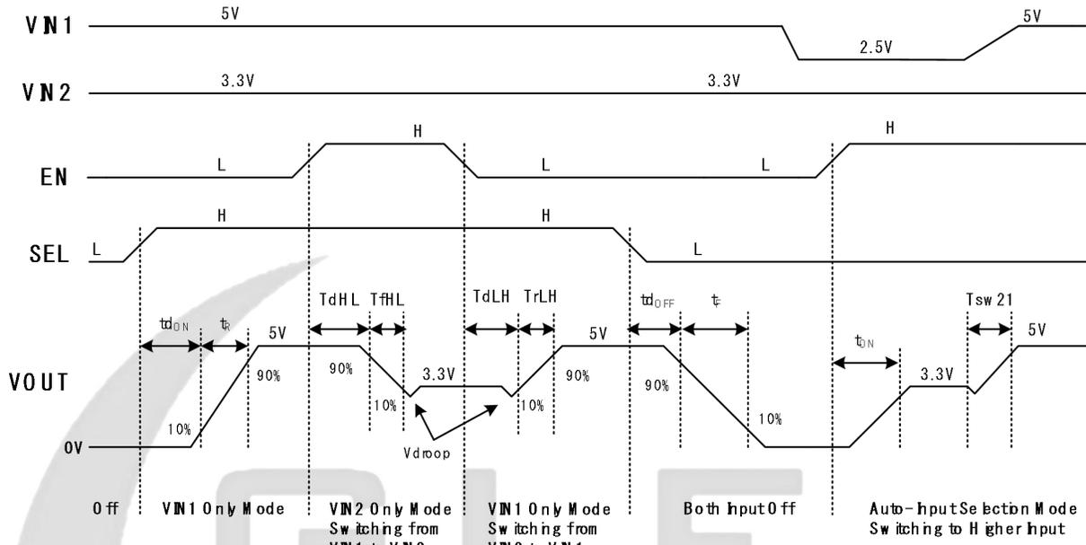
**Figure 3. Timing Diagram**
