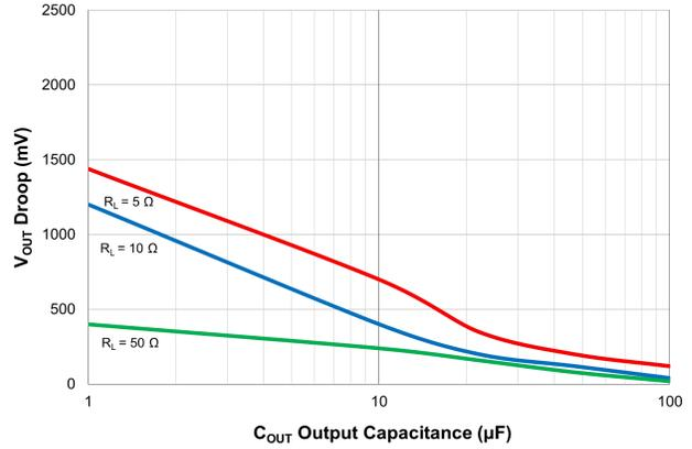
Figure 13. Output Voltage Droop at Switching Over from  $V_{IN2}$  (3.3V) to  $V_{IN1}$  (5V)
