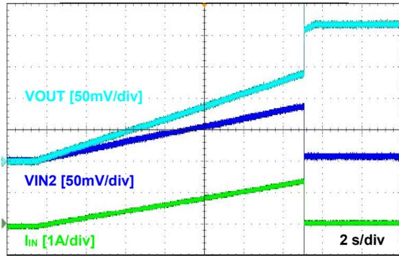
**Figure 18. True Reverse Current Blocking on Each VIN**
