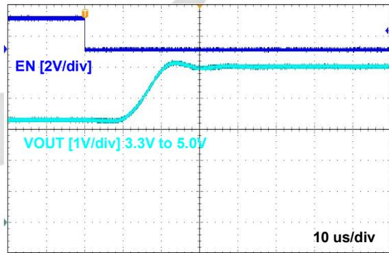
Figure 17.  $V_{OUT}$  Switchover 3.3  $V_{IN}$  to 5  $V_{IN}$
