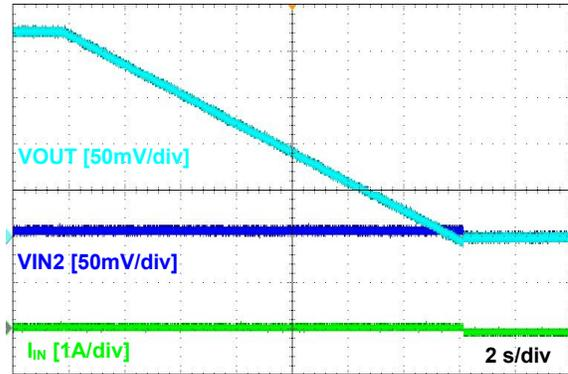
**Figure 19. True Reverse Current Blocking Release**
