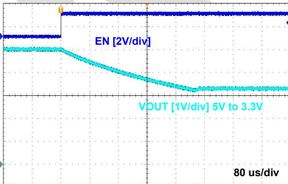
Figure 16.  $V_{OUT}$  Switchover from 5  $V_{IN}$  to 3.3  $V_{IN}$
