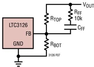
Figure 7. Feedforward Resistor ( $R_{FF}$ ) for Improved Noise Robustness
