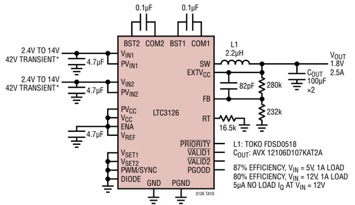
\*The step-down converter can operate over the specified input voltage range without any pulse skipping for loads from 250mA to 2.5A. However, in all applications, the converter can operate from an input voltage as high as 42V, but pulse skipping may occur if operated above the specified voltage range. Pulse skipping is not detrimental to the IC, but can result in significant output voltage ripple and is therefore generally avoided while in nominal operating conditions.
