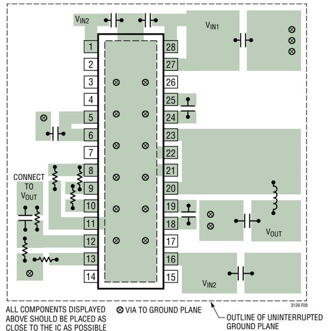
Figure 9. Recommended PC Board Layout for TSSOP Package
