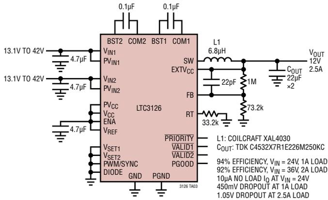
12V, 2MHz Step-Down Converter with Dual Inputs
