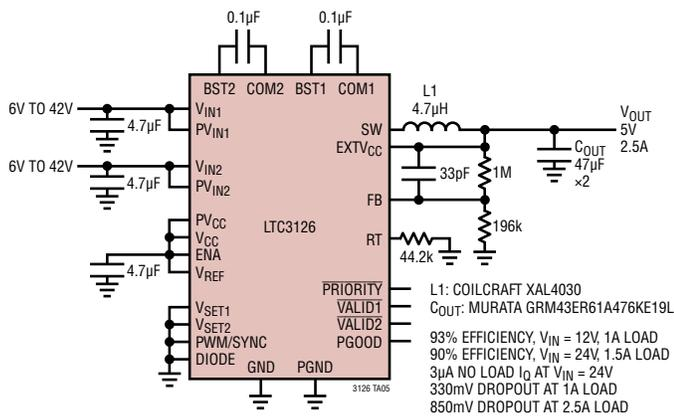
5V, 2MHz Step-Down Converter with Dual Inputs
