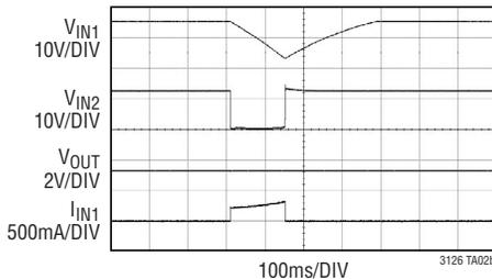
V<sub>OUT</sub> Hold-Up with Loss of Input Supply
