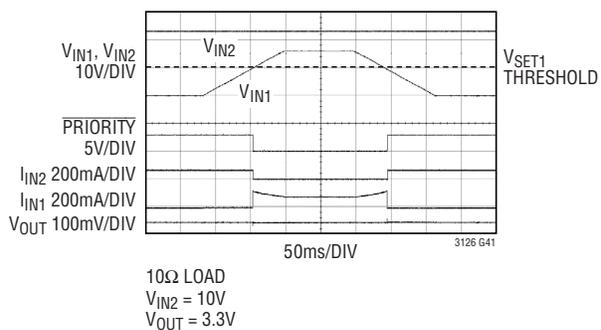
**Hot Plug of Automotive Input,  $V_{IN1}$**
