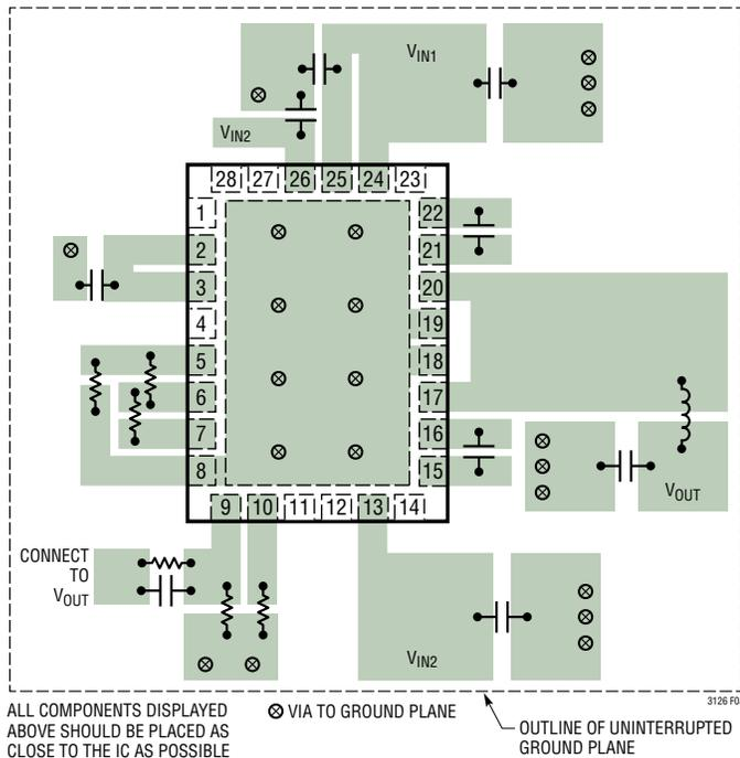
Figure 8. Recommended PC Board Layout for QFN Package
