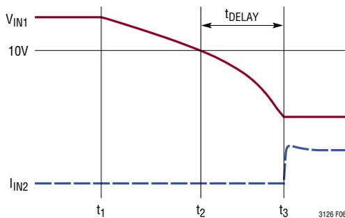
Figure 6. Waveforms During Transition from  $V_{\text{IN}1}$  to  $V_{\text{IN}2}$
