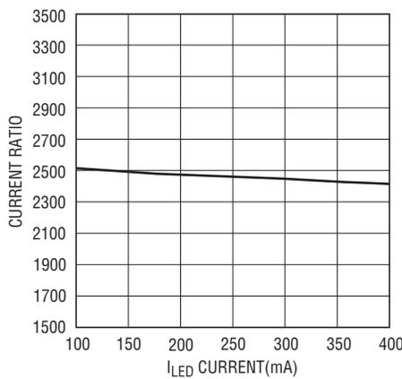
**Flash  $I_{LED}/I_{SET}$  Current Ratio vs  $I_{LED}$  Current (ENT = ENF = HIGH)**
