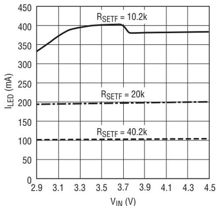
**Flash Mode  $I_{LED}$  Current vs  $V_{IN}$  (ENT = LOW, ENF = HIGH)**
