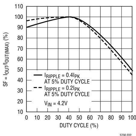
Figure 2. Maximum Output Current vs Duty Cycle
