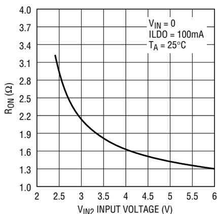
**PGOOD R<sub>ON</sub> vs Input Voltage**
