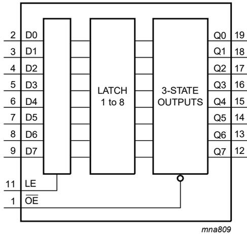
Fig. 3. Functional diagram
