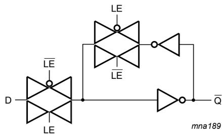
Fig. 4. Logic diagram (one latch)
