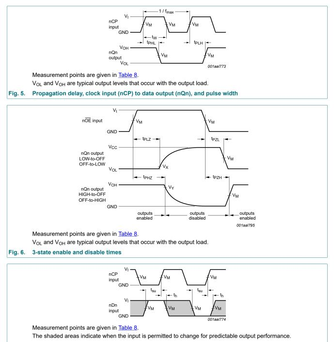
Fig. 7. Data setup and hold times for input (nDn) to input (nCP)
