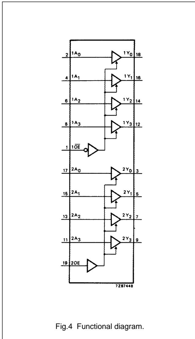
Fig.4 Functional diagram.
