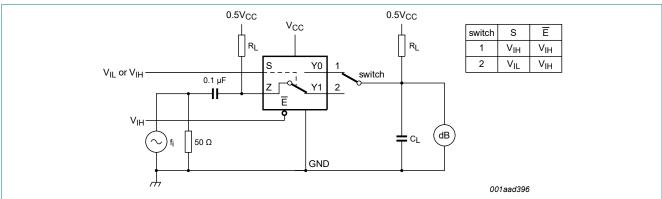
Adjust f<sub>i</sub> voltage to obtain 0 dBm level at input
