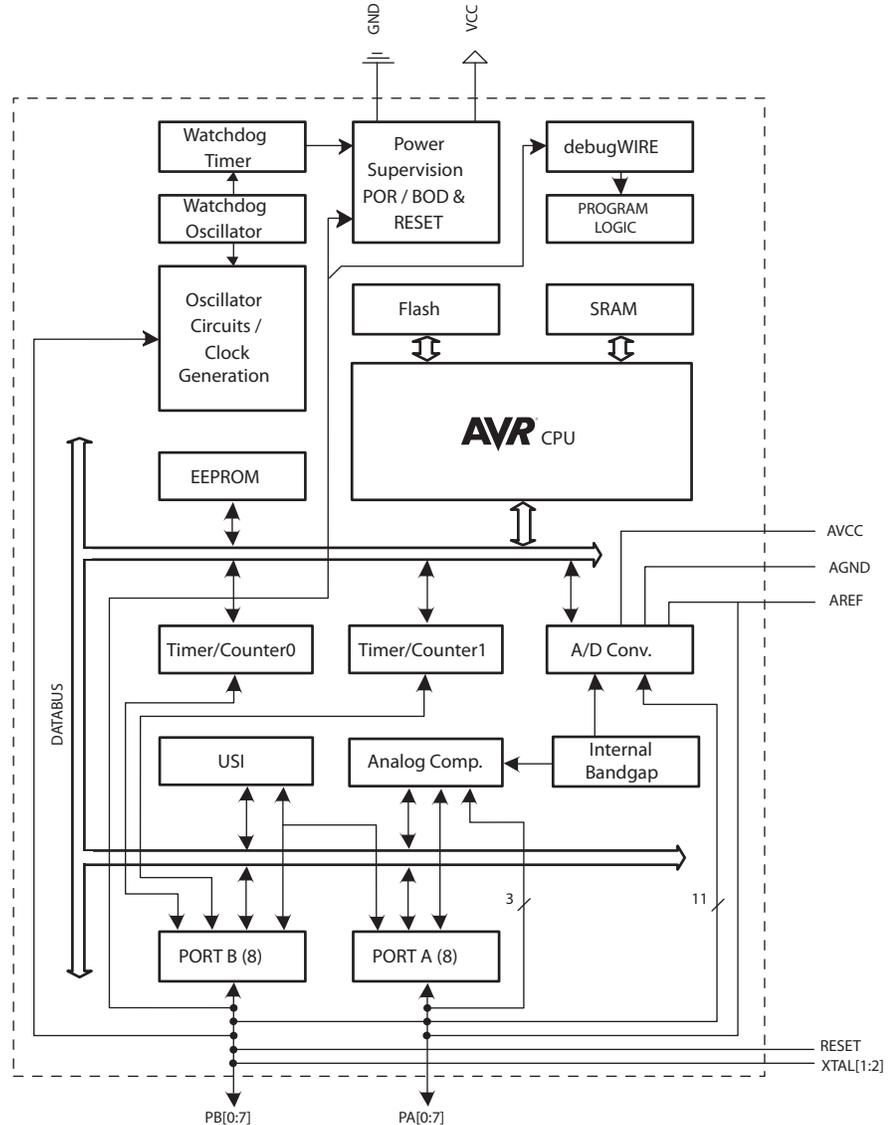
The AVR core combines a rich instruction set with 32 general purpose working registers. All 32 registers are directly connected to the Arithmetic Logic Unit (ALU), allowing two independent registers to be accessed in one single instruction executed in one clock cycle. The resulting architecture is more code efficient while achieving throughputs up to ten times faster than conventional CISC microcontrollers.
