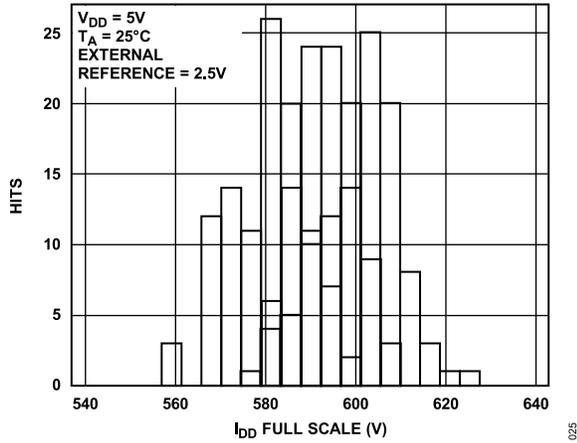
Figure 23.  $I_{DD}$  Histogram with External Reference
