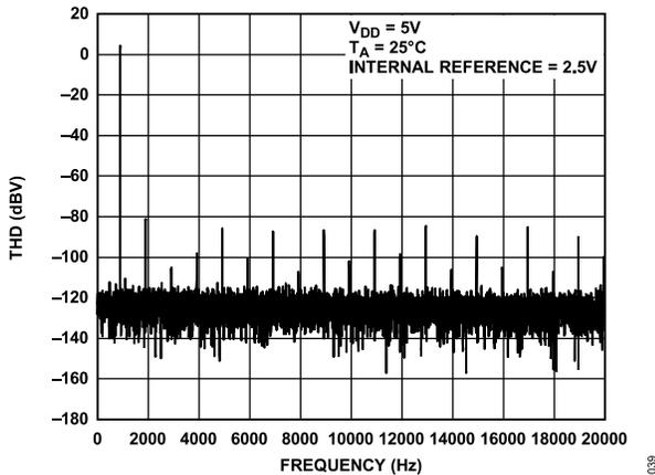
Figure 37. Total Harmonic Distortion at 1 kHz
