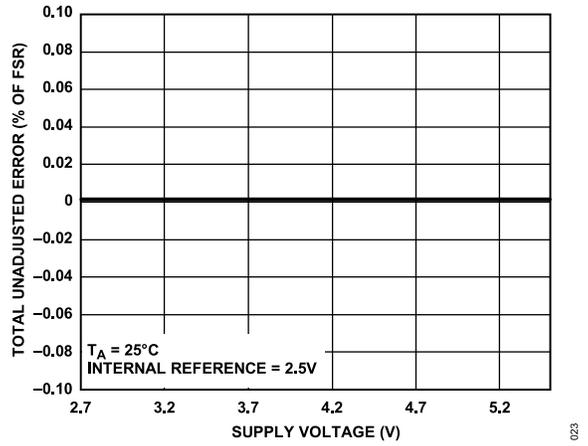
Figure 21. Total Unadjusted Error vs. Supply Voltage, Gain = 1
