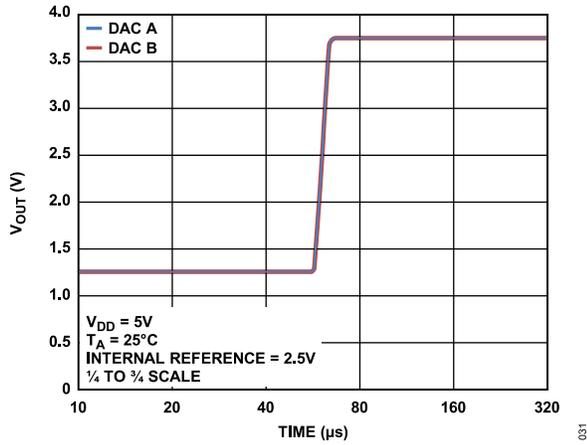
Figure 29. Settling Time
