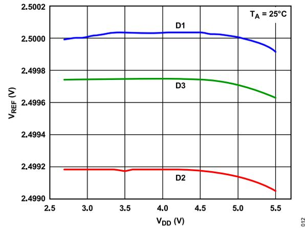
Figure 10. Internal Reference Voltage vs. Supply Voltage
