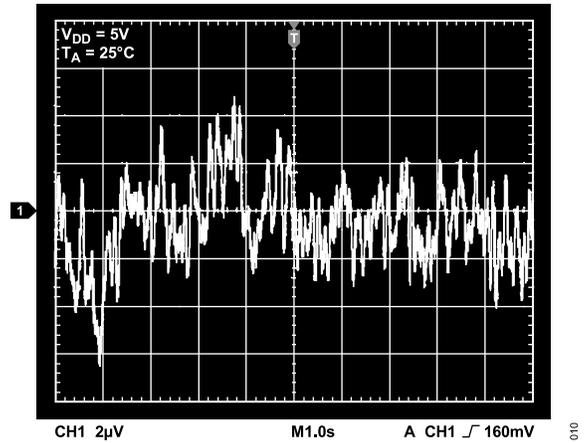
Figure 8. Internal Reference Noise, 0.1 Hz to 10 Hz
