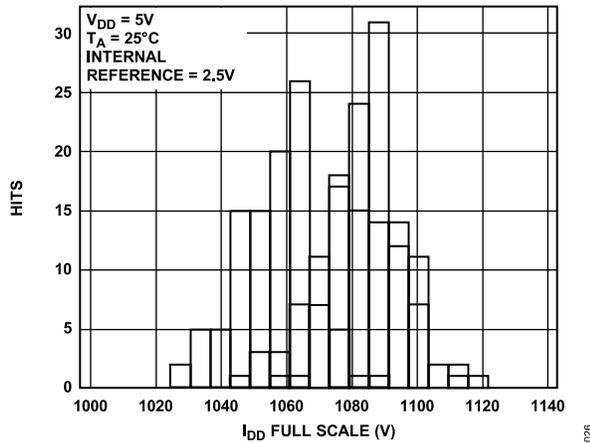
Figure 24.  $I_{DD}$  Histogram with Internal Reference,  $V_{REFOUT} = 2.5\text{ V}$ , Gain = 2
