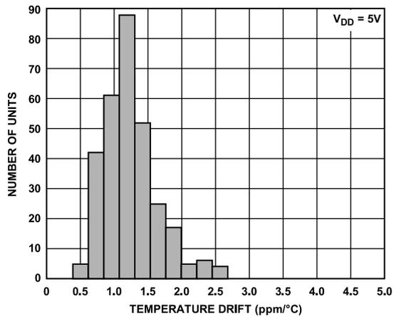
Figure 6. Reference Output Temperature Drift Histogram
