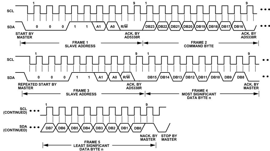
Figure 44. I<sup>2</sup>C Read Operation
