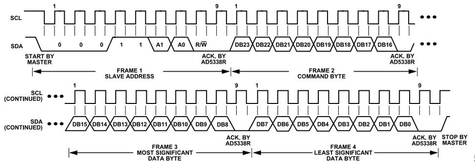
**Figure 43. I<sup>2</sup>C Write Operation**
