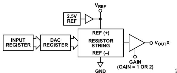
Figure 40. Single DAC Channel Architecture Block Diagram
