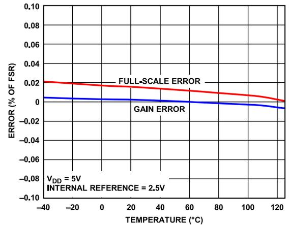
Figure 16. Gain Error and Full-Scale Error vs. Temperature
