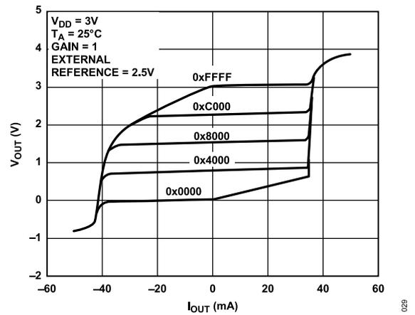
Figure 27. Source and Sink Capability at  $V_{DD} = 3\text{ V}$
