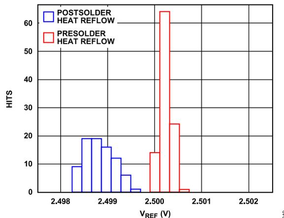
Figure 47. SHR Reference Voltage Shift
