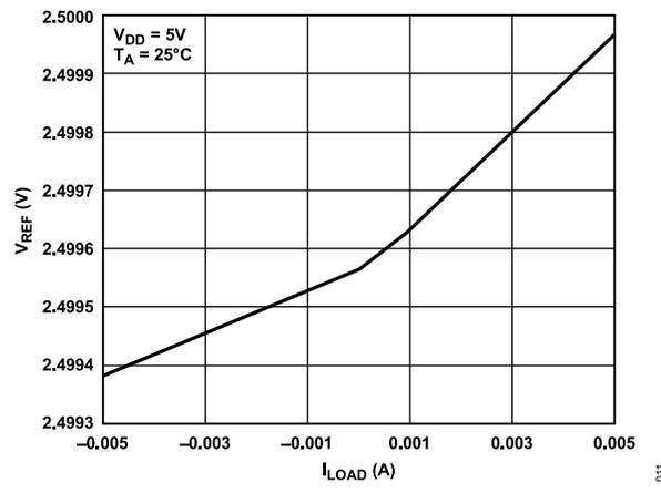
Figure 9. Internal Reference Voltage vs. Load Current
