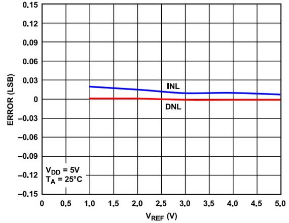
Figure 14. INL Error and DNL Error vs.  $V_{REF}$
