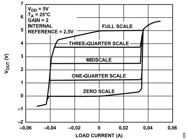
Figure 26. Source and Sink Capability at  $V_{DD} = 5\text{ V}$
