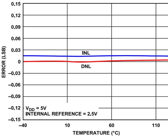
Figure 13. INL Error and DNL Error vs. Temperature
