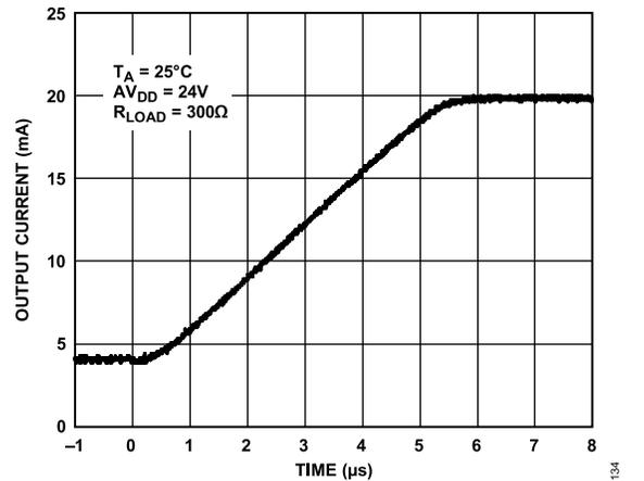
Figure 36. 4 mA to 20 mA Output Current Step
