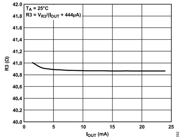
Figure 50. R<sub>3</sub> Resistor Value vs. I<sub>OUT</sub>
