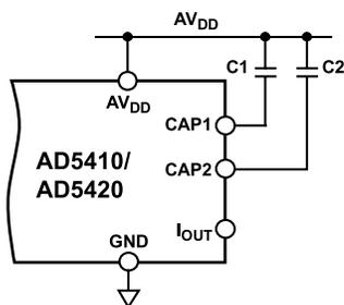
Figure 44. I<sub>OUT</sub> Filtering Capacitors
