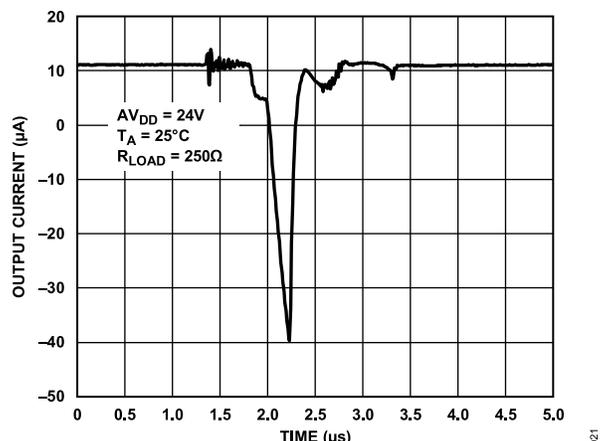
Figure 24. Output Current vs. Time on Output Enable
