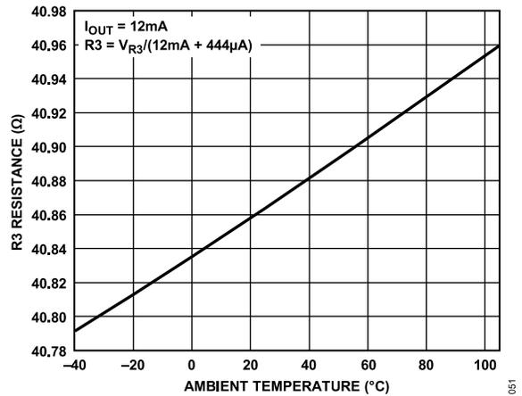
Figure 49. R<sub>3</sub> Resistor Value vs. Temperature
