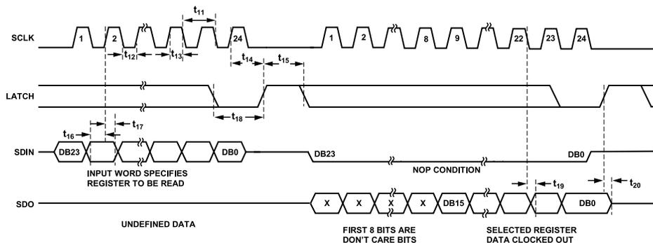
Figure 3. Readback Mode Timing Diagram
