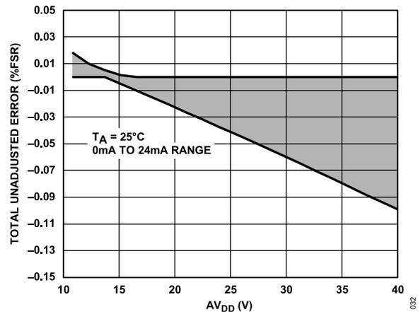
Figure 21. Total Unadjusted Error vs.  $AV_{DD}$ , Internal  $R_{SET}$
