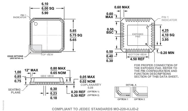
Figure 57. 40-Lead Lead Frame Chip Scale Package [LFCSP] 6 mm x 6 mm Body and 0.85 mm Package Height (CP-40-1)
