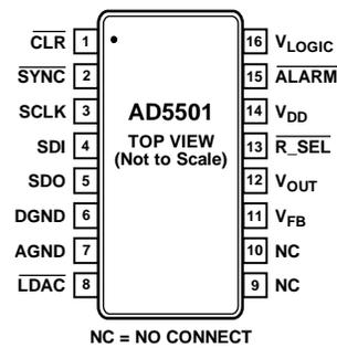
Figure 5. Pin Configuration
