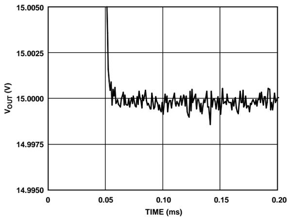
Figure 8. Output Settling Time (High to Low)
