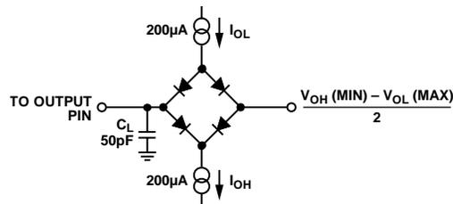
Figure 2. Load Circuit for SDO Timing Diagram
