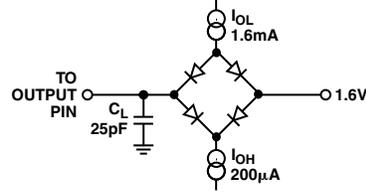
Figure 2. Load Circuit for Digital Output Timing Specifications
