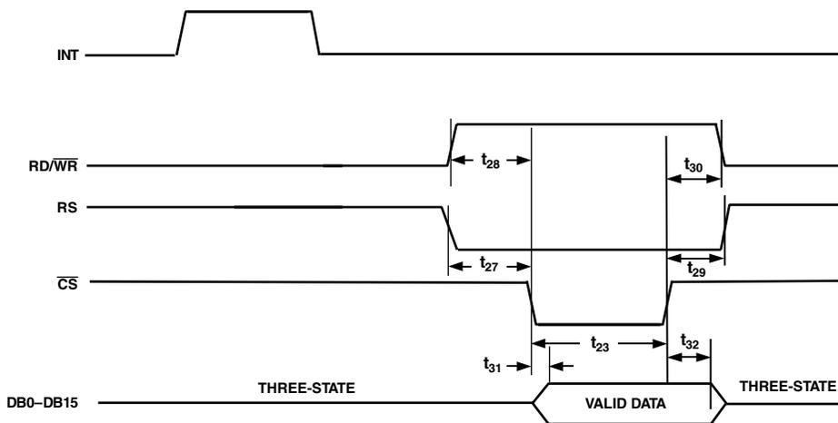
Figure 7. Parallel Mode (Reading Data from the AD7725)
