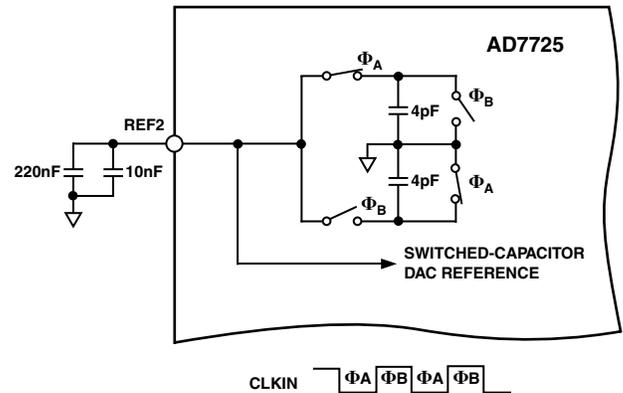
Figure 16. REF2 Equivalent Input Circuit
