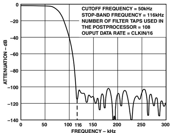
Figure 1. Digital Filter Characteristics Used for Specifications
