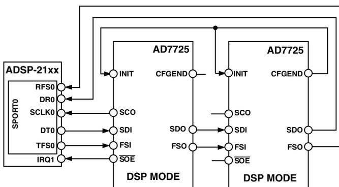
Figure 33. Daisy-Chaining Devices with a Common DSP
