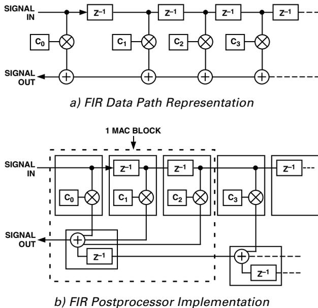
Figure 20. AD7725 Postprocessor Mapping
