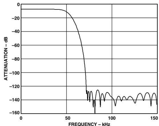
Figure 21. Default Filter Response for CLKIN = 9.6 MHz
