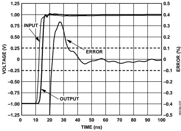
Figure 22. Settling Time (0.1%) at Various Loads
