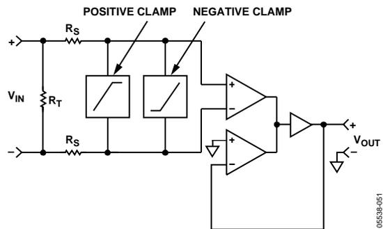
Figure 42. Differential-Mode Clamping
