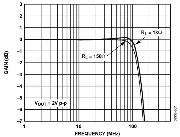
Figure 9. Large Signal Frequency Response at Various Loads
