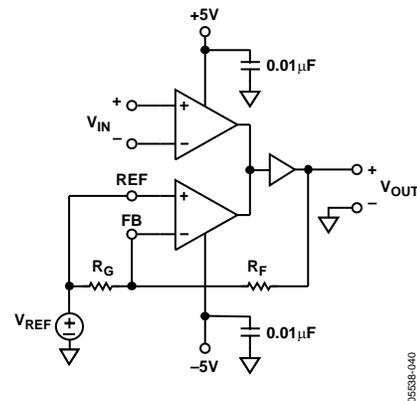
Figure 39. Basic Gain Circuit:  $V_{OUT} = V_{IN}(1 + R_F/R_G) + V_{REF}$
