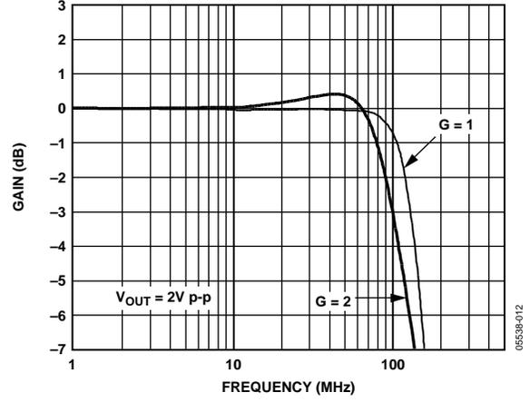
Figure 14. Large Signal Frequency Response at Various Gains
