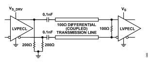
Figure 61. AC-Coupled LVPECL with Parallel Transmission Line
