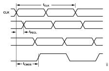
Figure 3. CLK/CLK to Clock Output Timing, DIV = 1
