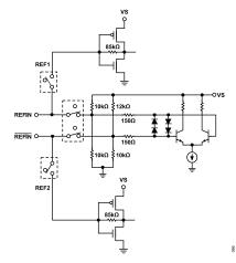
Figure 31. REFIN Equivalent Circuit for Non-XTAL Mode
