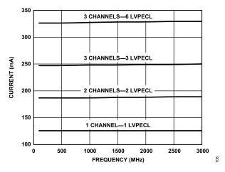
Figure 6. Total Current vs. Frequency, CLK-to-Output (PLL Off),LVPECL Outputs Terminated 50 Ω to V<sub>S DRV</sub> - 2 V
