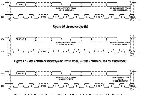
Figure 48. Data Transfer Process (Main Read Mode, 2-Byte Transfer Used for Illustration)
