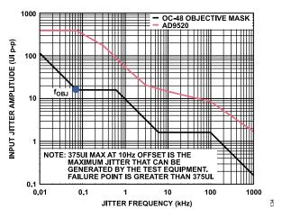
Figure 25. Telcordia GR-253 Jitter Tolerance Plot
