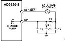
Figure 30. Example of External Loop Filter for PLL
