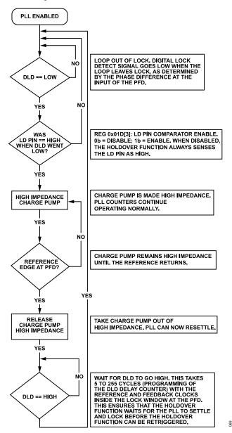
Figure 35. Flowchart of Automatic/Internal Holdover Mode
