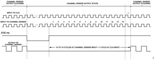
Figure 41. SYNC Timing Pipeline Delay When the VCO Divider Is Not Used
