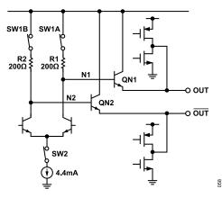
Figure 42. LVPECL Output Simplified Equivalent Circuit
