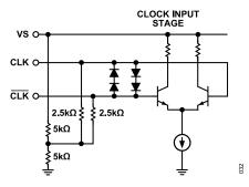
Figure 34. CLK Equivalent Input Circuit
