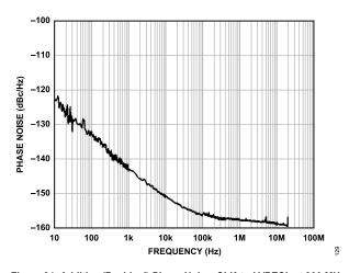
Figure 21. Additive (Residual) Phase Noise, CLK-to-LVPECL at 200 MHz, Divide-by-5
