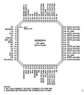
Figure 5. Pin Configuration
