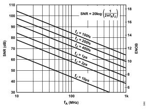
Figure 58. SNR and ENOB vs. Analog Input Frequency
