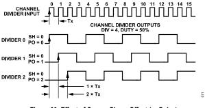
Figure 39. Effect of Coarse Phase Offset (or Delay)
