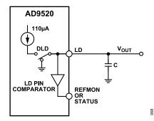
Figure 33. Current Source Digital Lock Detect
