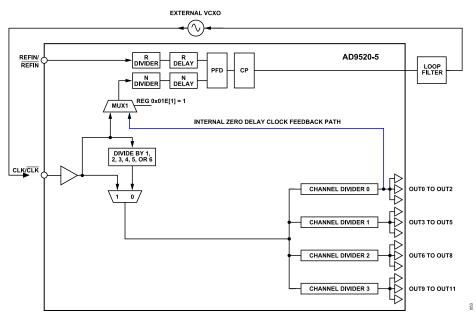
Figure 37. Zero Delay Function
