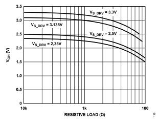
Figure 12. CMOS Output V<sub>OH</sub> (Static) vs. R<sub>LOAD</sub> (to Ground)
