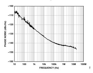
Figure 20. Additive (Residual) Phase Noise, CLK-to-LVPECL at 1600 MHz, Divide-by-1
