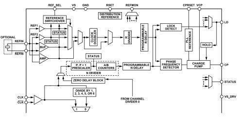
Figure 29. PLL Functional Block Diagram
