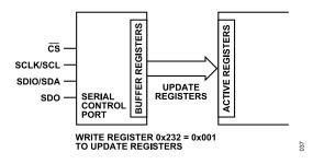
Figure 51. Relationship Between Serial Control Port Buffer Registers and Active Registers of the AD9520-5
