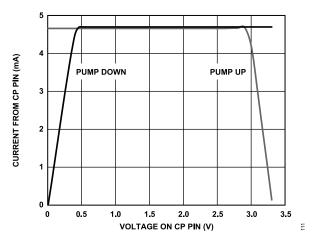
Figure 8. Charge Pump Characteristics at CP<sub>V</sub>= 3.3 V
