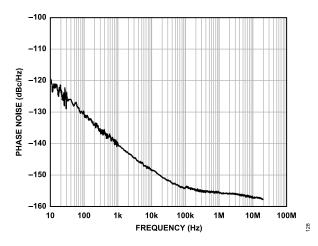
Figure 19. Additive (Residual) Phase Noise, CLK-to-LVPECL at 245.76 MHz, Divide-by-1
