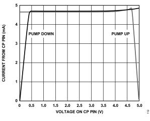
Figure 9. Charge Pump Characteristics at  $CP_V = 5.0 V$
