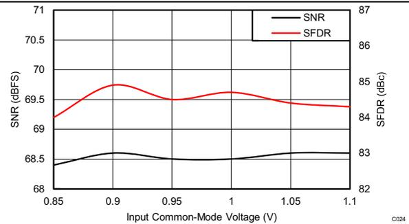
Figure 123. Performance vs Input Common-Mode Voltage (170 MHz)
