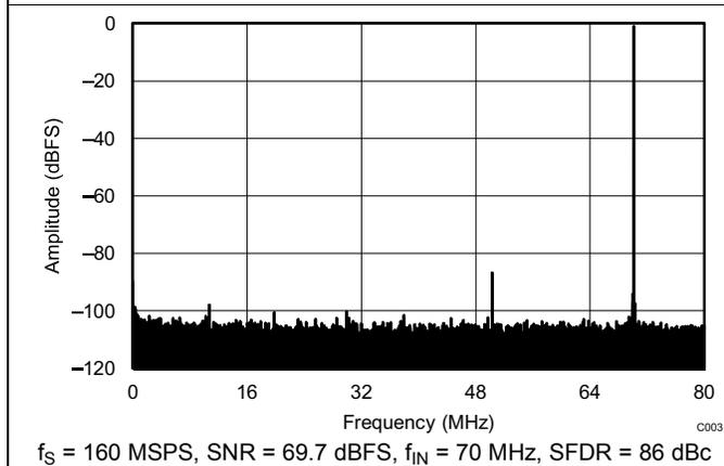
Figure 3. FFT for 70-MHz Input Signal (Dither On)
