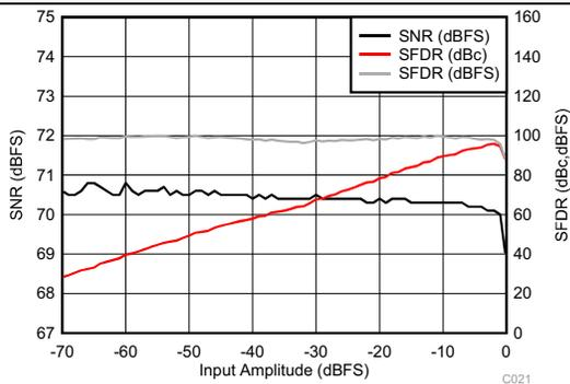
Figure 54. Performance vs Input Amplitude (30 MHz)
