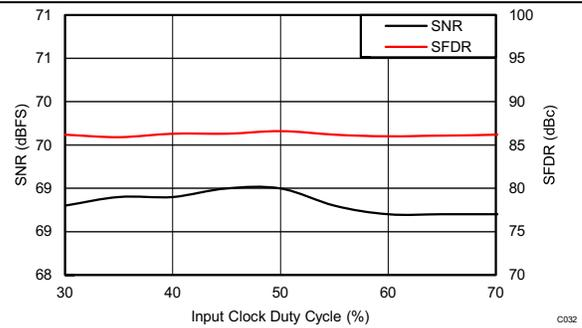
**Figure 98. Performance vs Clock Duty Cycle (150 MHz)**
