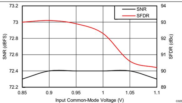
Figure 56. Performance vs Input Common-Mode Voltage (30 MHz)
