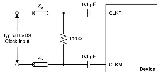
**Figure 148. Differential Sine-Wave Clock Driving Circuit**
