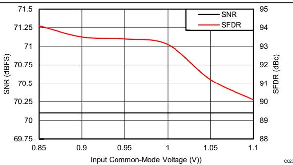
**Figure 89. Performance vs Input Common-Mode Voltage (30 MHz)**
