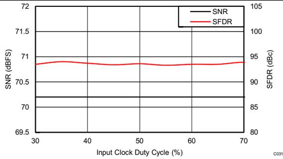
**Figure 64. Performance vs Clock Duty Cycle (40 MHz)**
