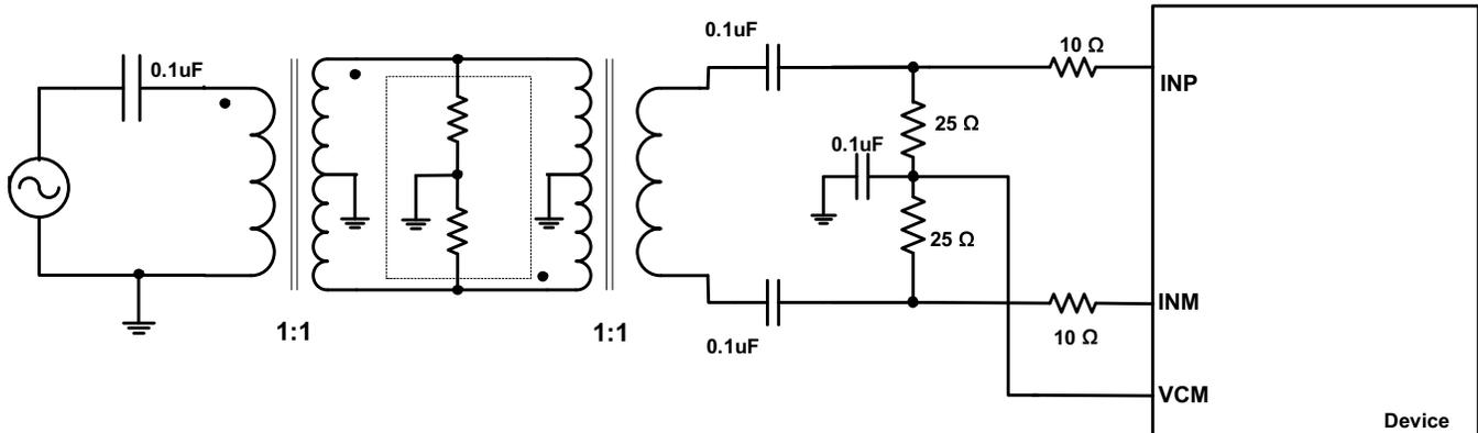
Figure 206. Driving Circuit for High Input Frequencies ( $f_{IN} > 230$  MHz)
