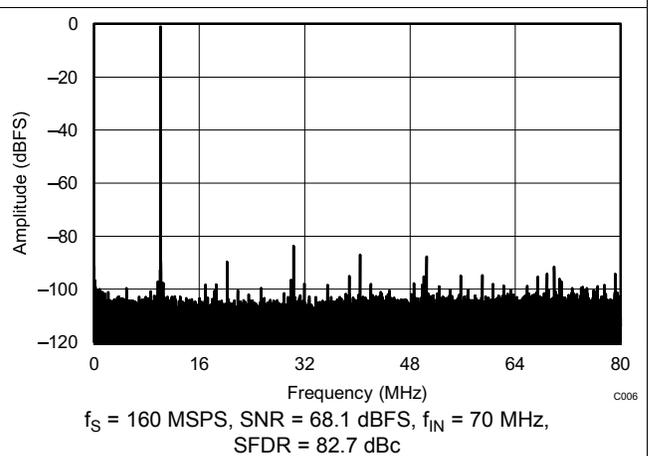
Figure 6. FFT for 170-MHz Input Signal (Dither Off)
