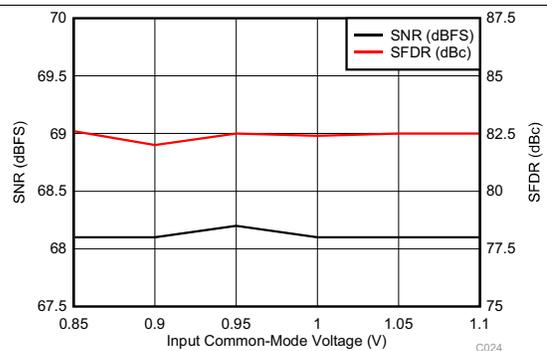
**Figure 24. Performance vs Input Common-Mode Voltage (170 MHz)**
