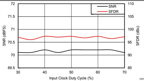
**Figure 97. Performance vs Clock Duty Cycle (40 MHz)**
