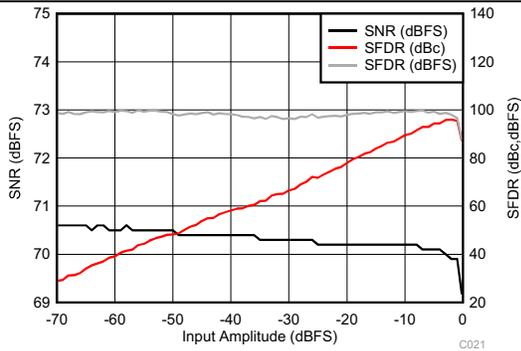
**Figure 87. Performance vs Input Amplitude (30 MHz)**
