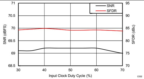
**Figure 65. Performance vs Clock Duty Cycle (150 MHz)**
