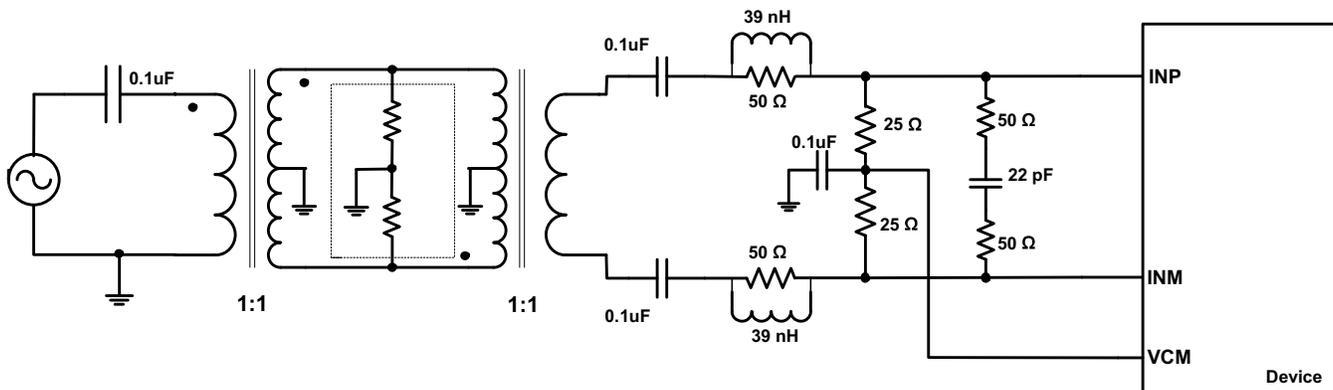
Figure 202. Driving Circuit for Low Input Frequencies
