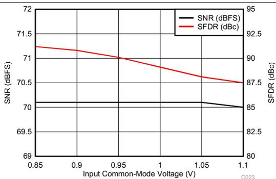
**Figure 23. Performance vs Input Common-Mode Voltage (30 MHz)**
