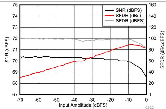
Figure 55. Performance vs Input Amplitude (170 MHz)
