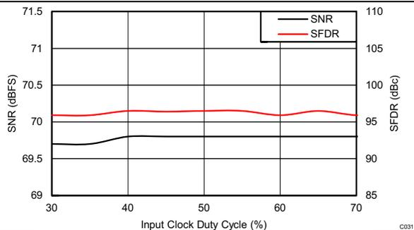
**Figure 130. Performance vs Clock Duty Cycle (40 MHz)**
