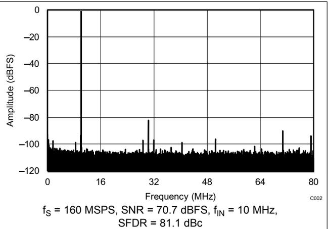
Figure 2. FFT for 10-MHz Input Signal (Dither Off)
