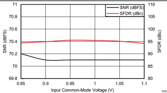
Figure 122. Performance vs Input Common-Mode Voltage (30 MHz)
