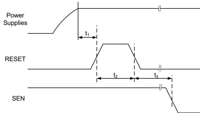
**Figure 164. Initialization of Serial Registers after Power-Up**
