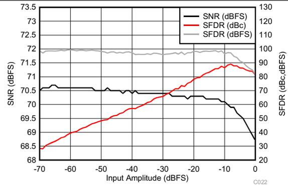
Figure 121. Performance vs Input Amplitude (170 MHz)
