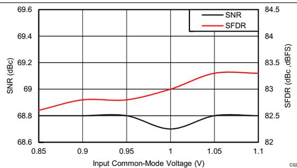
Figure 57. Performance vs Input Common-Mode Voltage (170 MHz)
