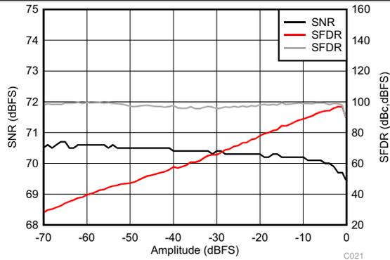
Figure 120. Performance vs Input Amplitude (30 MHz)
