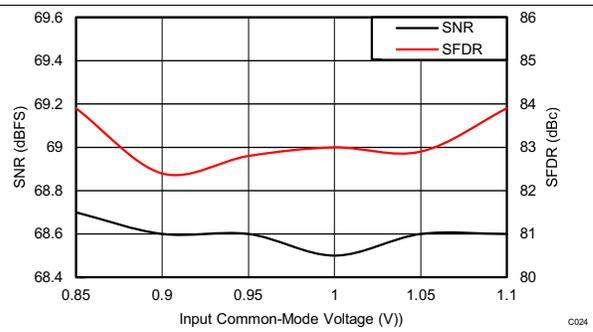
**Figure 90. Performance vs Input Common-Mode Voltage (170 MHz)**
