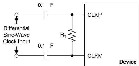
NOTE:  $R_T$  = termination resistor, if necessary.
