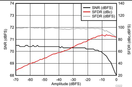
**Figure 22. Performance vs Input Amplitude (170 MHz)**
