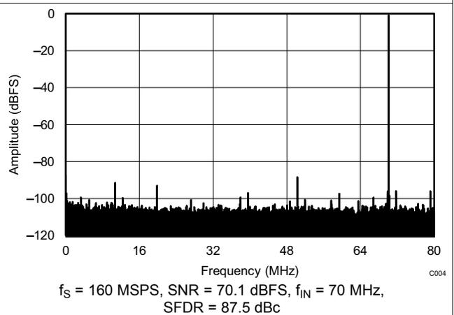
Figure 4. FFT for 70-MHz Input Signal (Dither Off)
