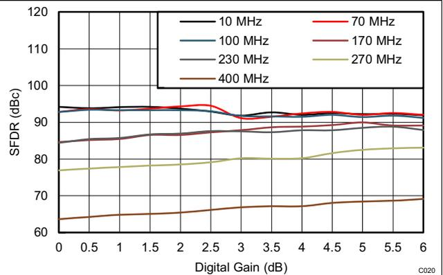
Figure 53. Spurious-Free Dynamic Range vs Digital Gain and Input Frequency
