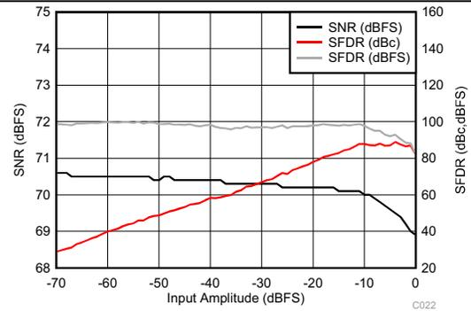
**Figure 88. Performance vs Input Amplitude (170 MHz)**
