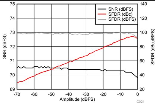
**Figure 21. Performance vs Input Amplitude (30 MHz)**
