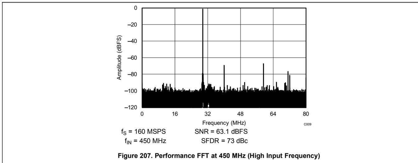
Figure 207. Performance FFT at 450 MHz (High Input Frequency)
