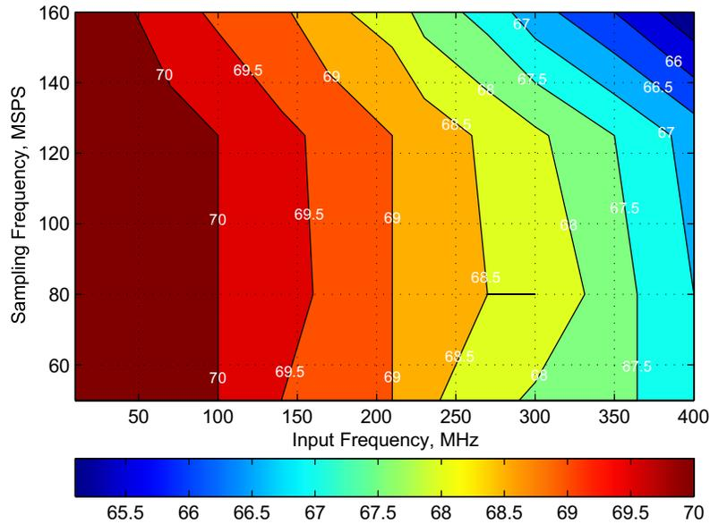
**Figure 141. Signal-to-Noise Ratio (SNR) for 0-dB Gain**
