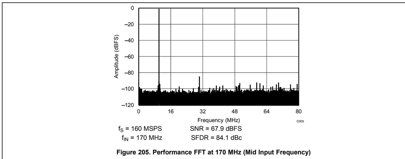
Figure 205. Performance FFT at 170 MHz (Mid Input Frequency)
