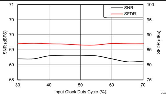
**Figure 131. Performance vs Clock Duty Cycle (150 MHz)**
