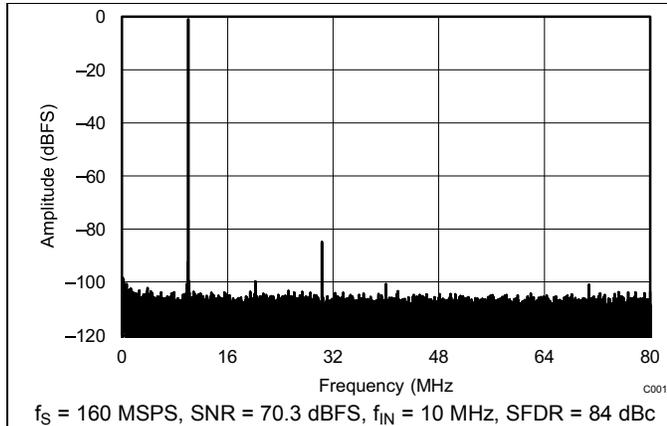
Figure 1. FFT for 10-MHz Input Signal (Dither On)
