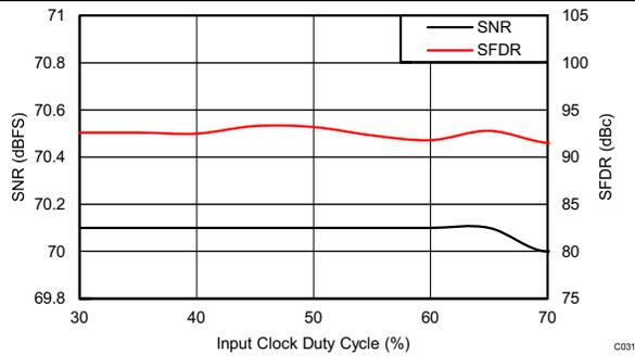
**Figure 31. Performance vs Clock Duty Cycle (40 MHz)**
