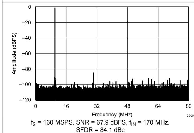
Figure 5. FFT for 170-MHz Input Signal (Dither On)
