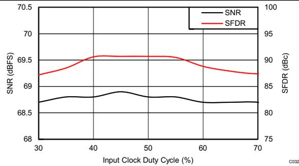
**Figure 32. Performance vs Clock Duty Cycle (150 MHz)**
