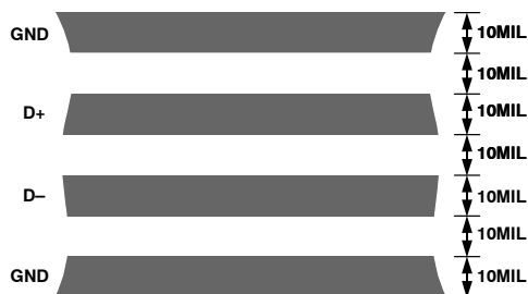
Figure 19. Arrangement of Signal Tracks
