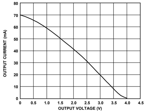
Figure 19. Output Current vs. Driver Differential Output Voltage
