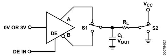
Figure 8. Driver Voltage Measurement Test Circuit 2
