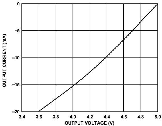
Figure 16. Output Current vs. Receiver Output High Voltage
