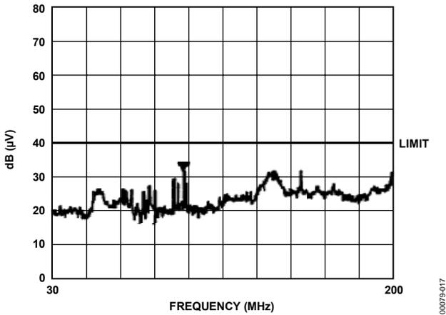
Figure 22. Radiated Emissions
