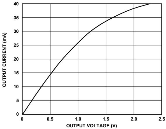
Figure 15. Output Current vs. Receiver Output Low Voltage
