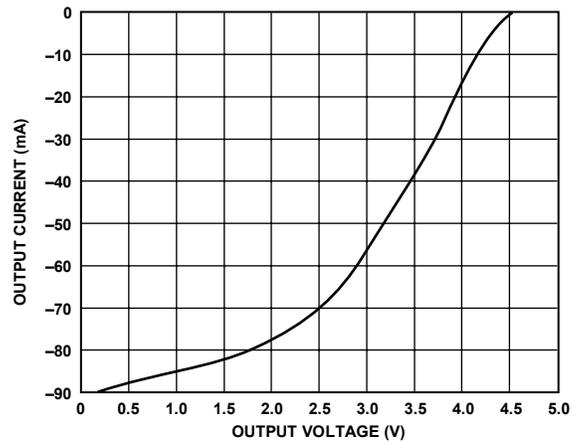
Figure 18. Output Current vs. Driver Output High Voltage
