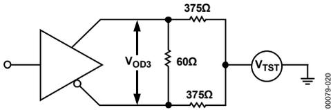
Figure 7. Driver Enable/Disable Test Circuit
