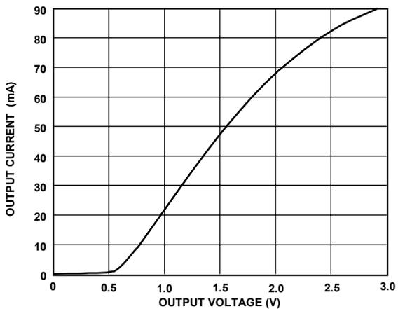
Figure 17. Output Current vs. Driver Output Low Voltage
