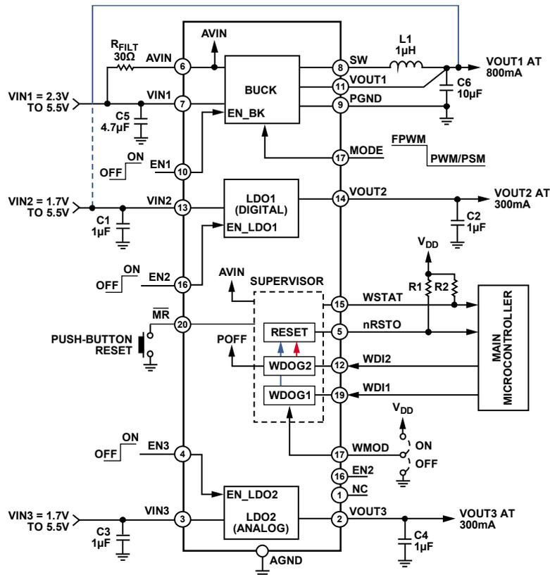
Figure 69. Application Diagram
