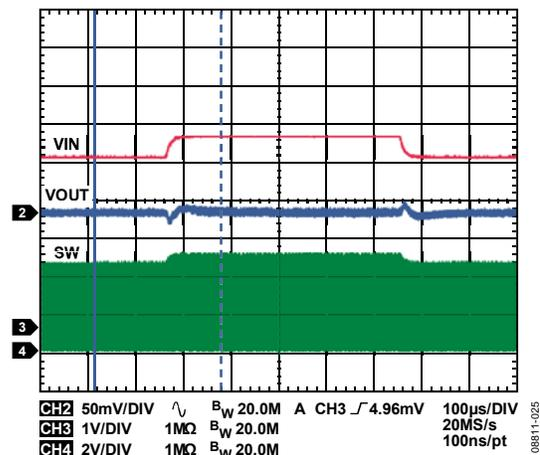
Figure 25. Buck Response to Line Transient, V<sub>IN</sub> = 4.5 V to 5.0 V, VOUT1 = 1.8 V, PWM Mode
