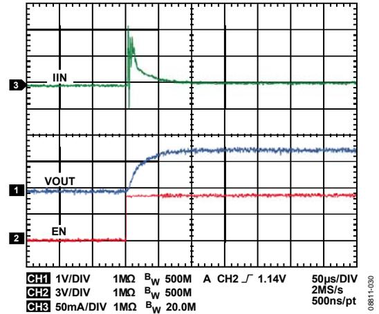
Figure 30. LDO1 Startup, VOUT3 = 1.5 V, IOUT3 = 5 mA
