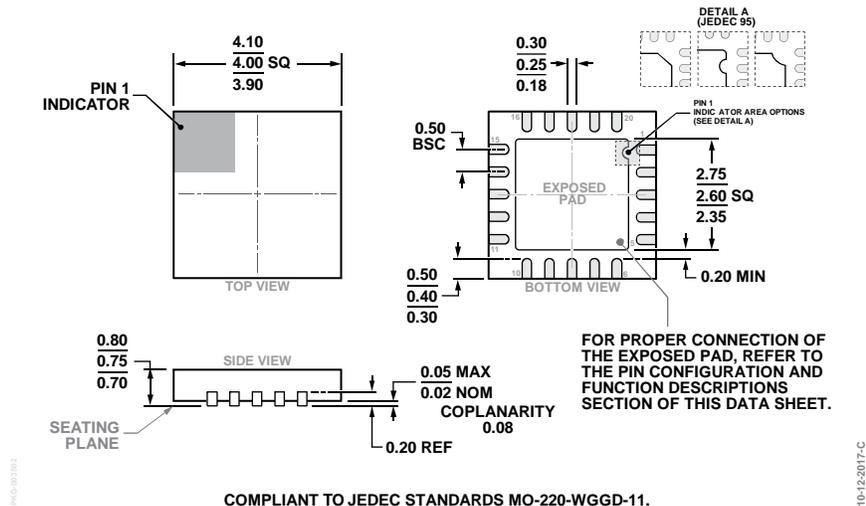
Figure 70. 20-Lead, Lead Frame Chip Scale Package [LFCSP]
