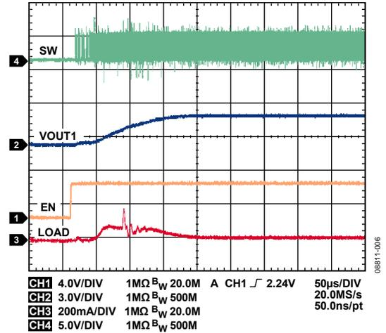
Figure 6. Buck Startup, VOUT1 = 1.8 V, IOUT2 = 20 mA
