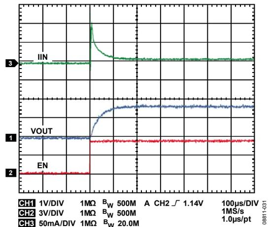
Figure 31. LDO2 Startup, VOUT3 = 3.3 V, IOUT3 = 5 mA
