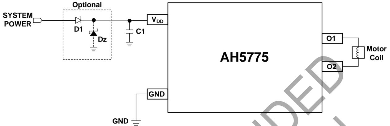
Note: 4. C1 is for power stabilization and to strengthen the noise immunity, the recommended capacitance is 0.1µF for small motor current to 1µF or higher for larger motor current and place capacitor as close to the V<sub>DD</sub> pin as possible. The value of C1 should be selected adequately to support the motor current.
