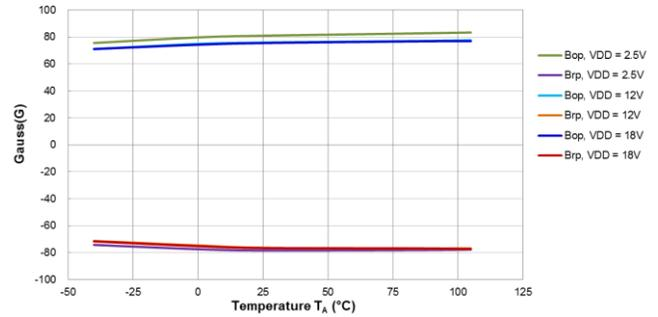
Magnetic Switch Points Bop & Brp vs. Temperature
