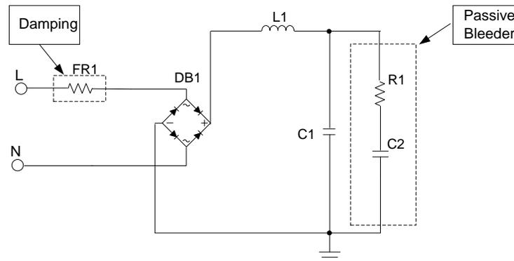
Figure 3. LED Driver Schematic with Passive Bleeder
