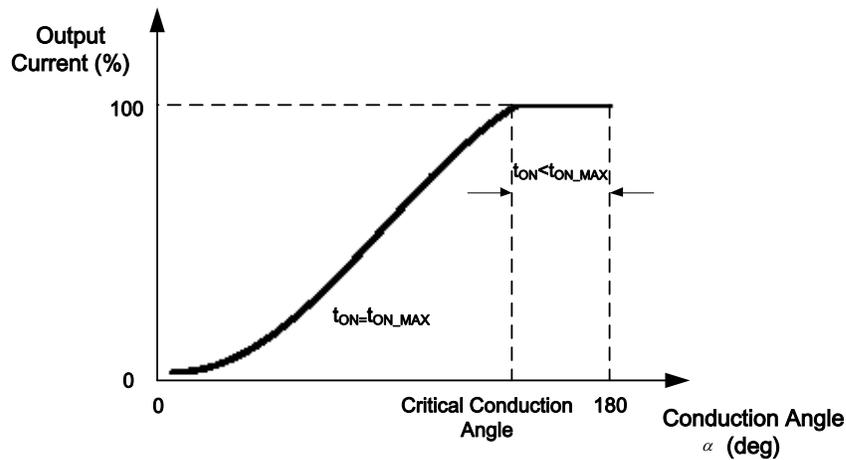
Figure 2. Dimming Curve
