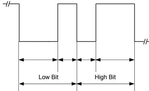
Figure 6. Single Wire Digital Dimming - Bit Coding
