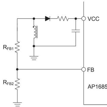
Figure 3. OVP Circuit
