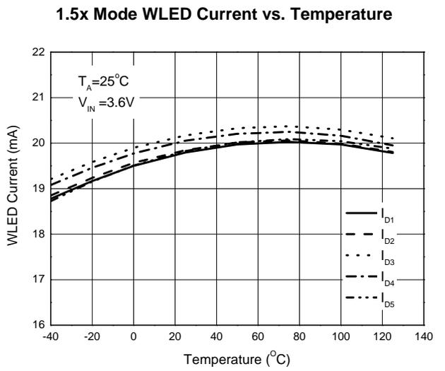
**Performance Characteristics** (Cont.  $T_A=+25^\circ\text{C}$ ,  $C_{IN}=C_1=C_2=C_{OUT}=1\mu\text{F}$ ,  $V_F=3.2\text{V}$ , unless otherwise noted.)
