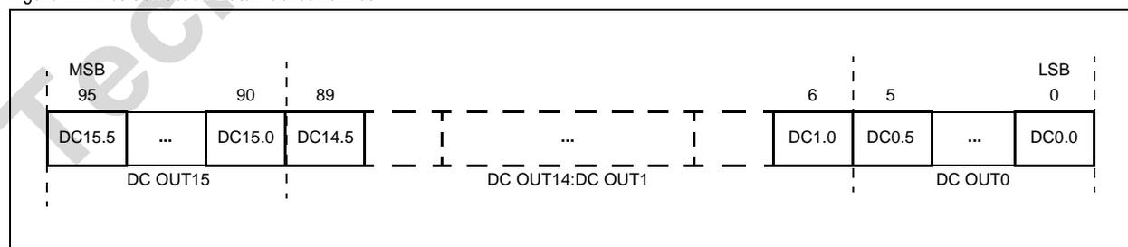
Figure 12. Dot Correction Data Input Timing Diagram
