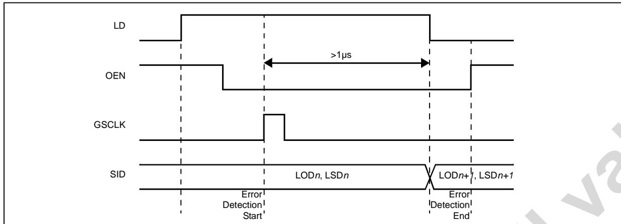
**Note:** The rising edge of LD latches new data into the internal registers depending on the logic level of the pin MODE. If the pin MODE is tied GND, the greyscale registers are updated. If the pin MODE is tied to VCC, the dot correction registers are updated.
