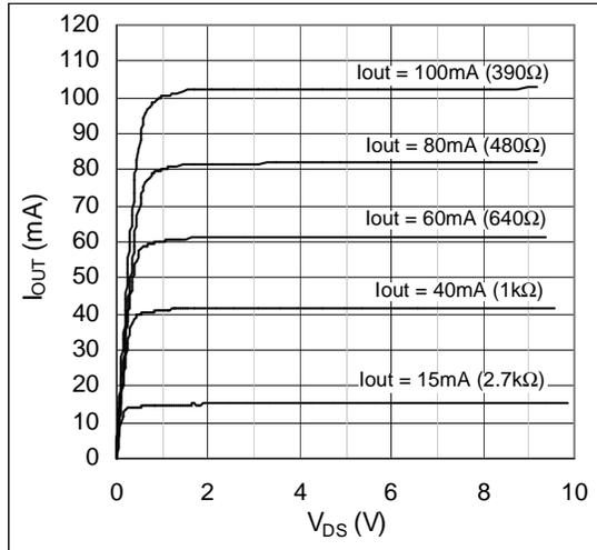
Figure 4. Output Current vs.  $V_{DS}$ ;  $V_{DD} = 5\text{V}$
