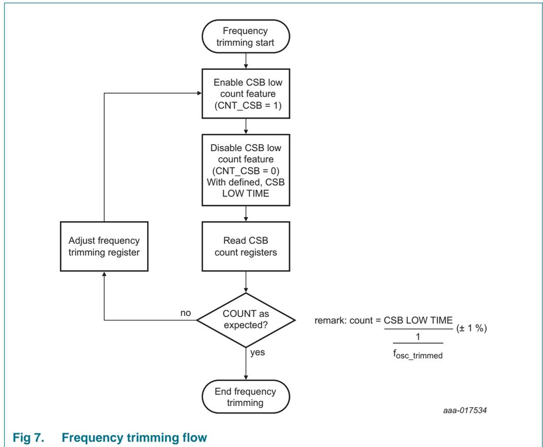
Fig 7. Frequency trimming flow
