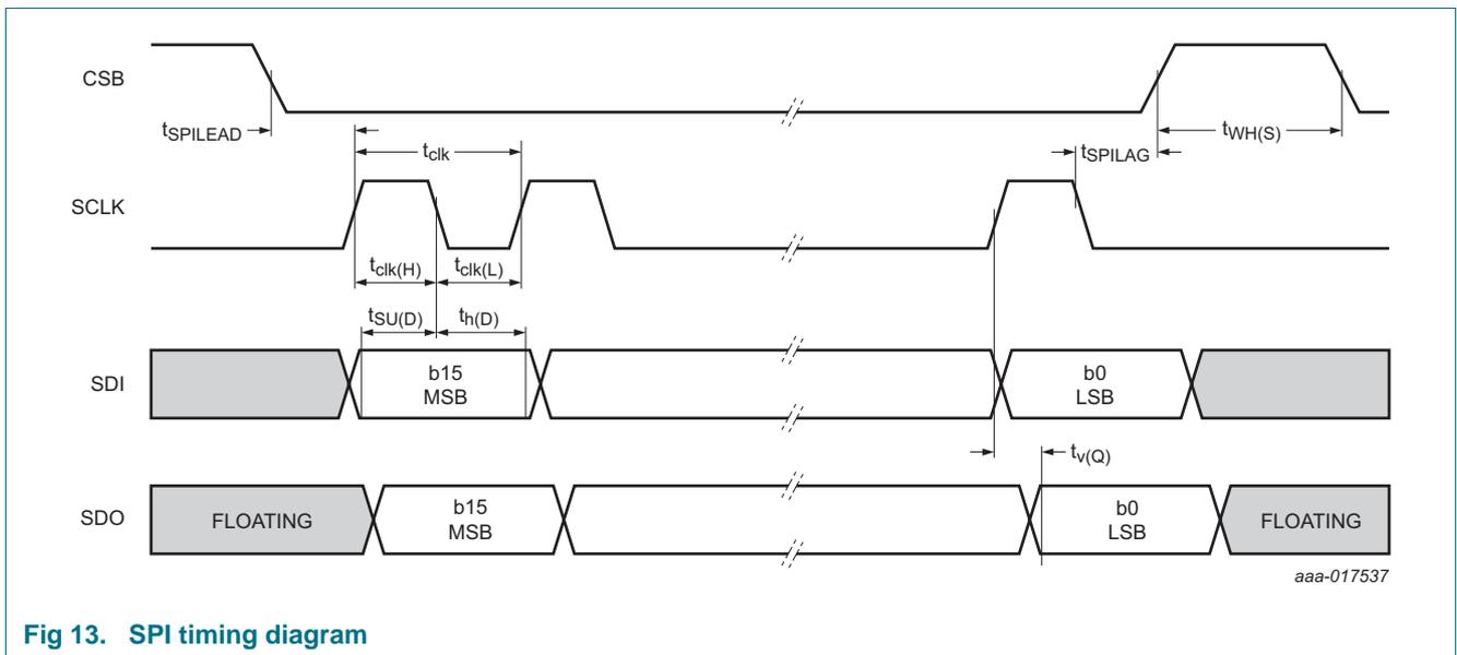
**Fig 13. SPI timing diagram**
