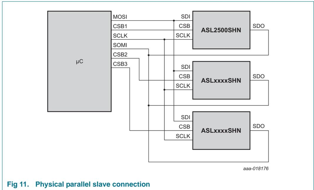
**Fig 11. Physical parallel slave connection**
