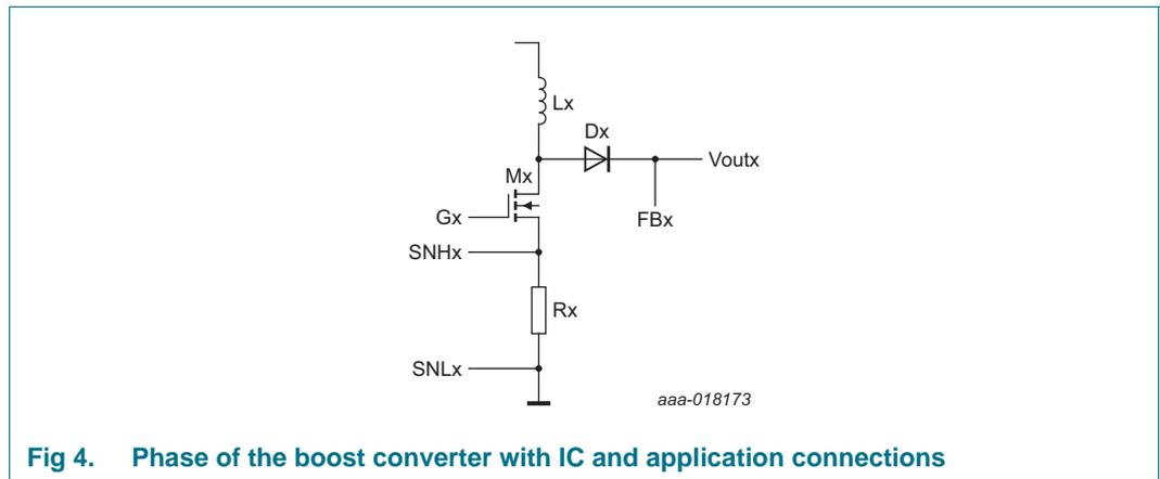
**Fig 4. Phase of the boost converter with IC and application connections**
