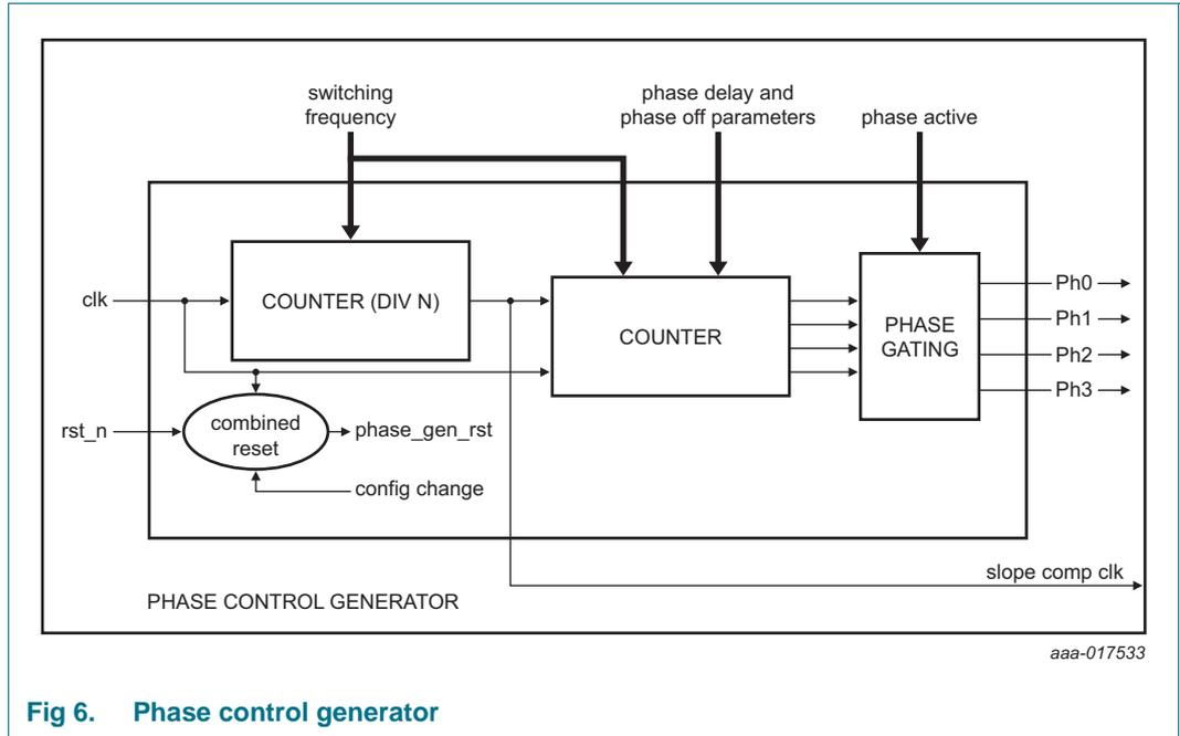
Fig 6. Phase control generator
