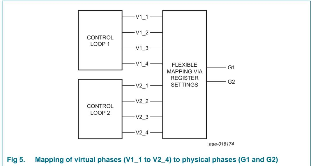
Fig 5. Mapping of virtual phases (V1\_1 to V2\_4) to physical phases (G1 and G2)
