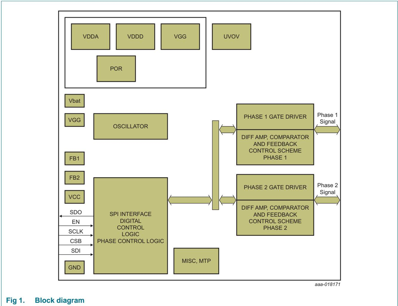
Fig 1. Block diagram
