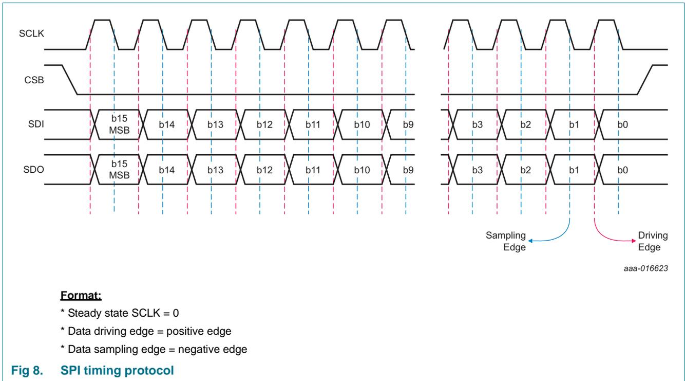
The data bits of the ASL2500SHN are arranged in registers of one-byte length. Each register is assigned to a 7-bit address. For writing into a register, 2 bytes must be sent to the LED driver. The first byte is an identifier byte that consists of the 7-bit address and one read-only bit. For writing, the read-only bit must be set to 0. The second byte is the data that is written into the register. So an SPI access consists of at least 16 bit.
