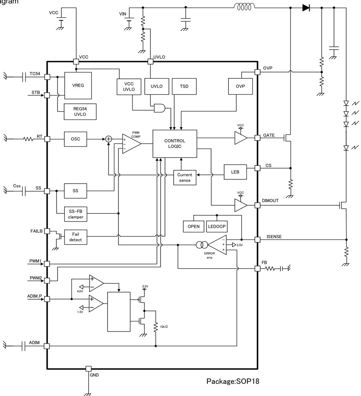
Figure 5. Block diagram
