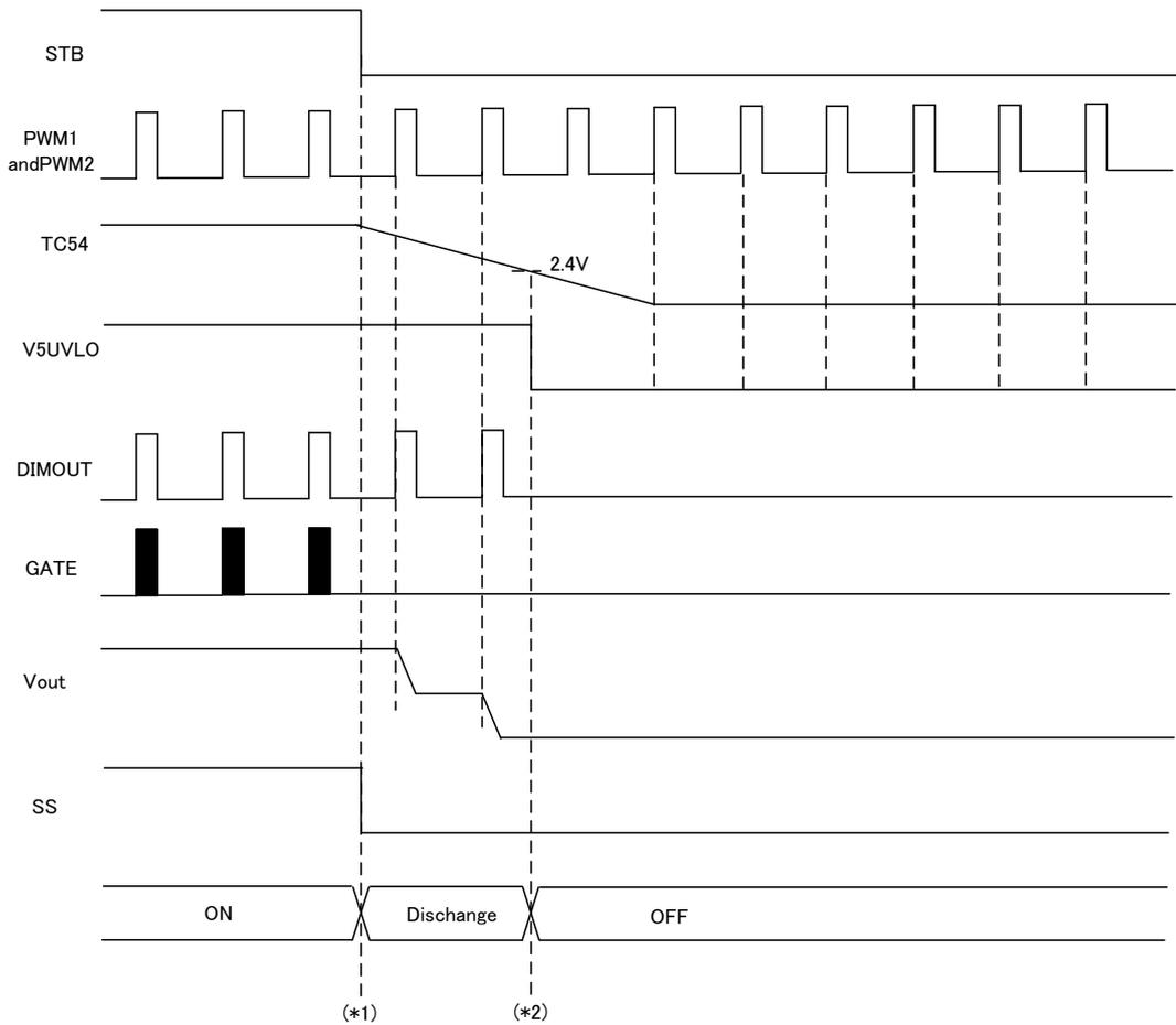
(\*1)...As STB pin turns High to Low, BD9488F stops the boost operation, starts the discharge of TC54.
