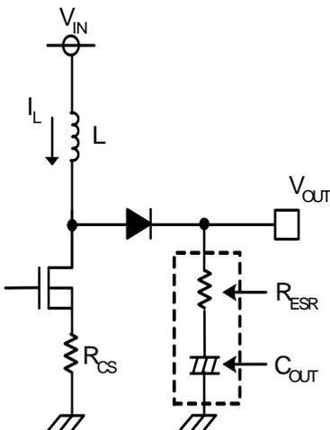
Output capacitor needs to be selected in consideration of equivalent series resistance required to even the stable area of output voltage or ripple voltage. Be aware that set LED current may not be flown due to decrease in LED terminal voltage if output ripple component is high. Output ripple voltage ΔVOUT is determined by Equation (4):
