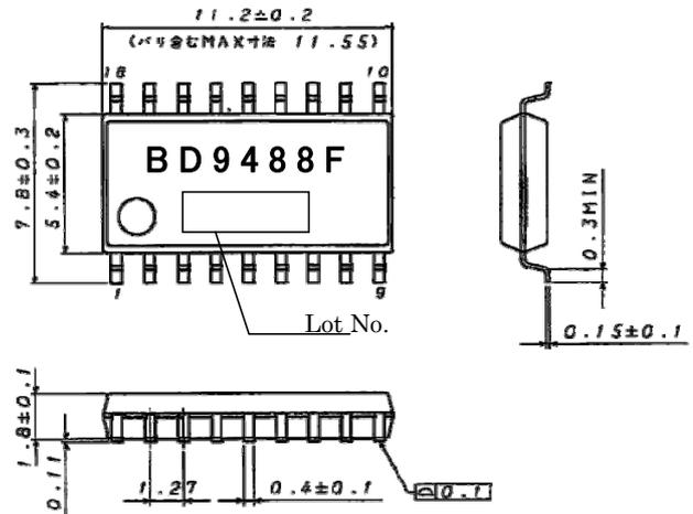
Figure 3-1. Pin configuration
