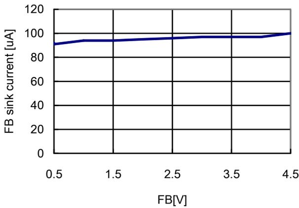
Figure 8. FB sink current vs FB voltage
