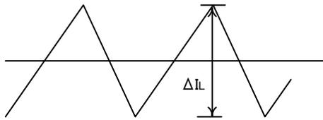
The inductor value affects the input ripple current. The equality in the section 3.5.1 is as following.
