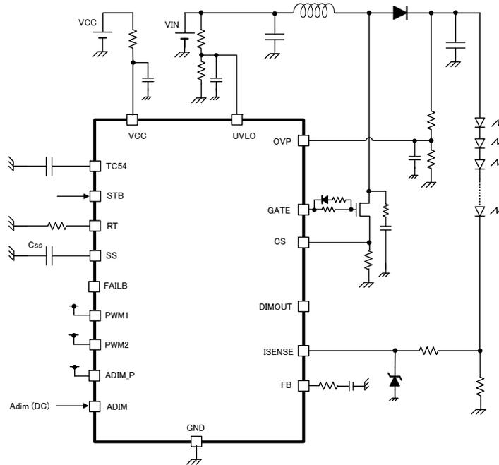
Figure 19. the circuit example of analog dimming only
