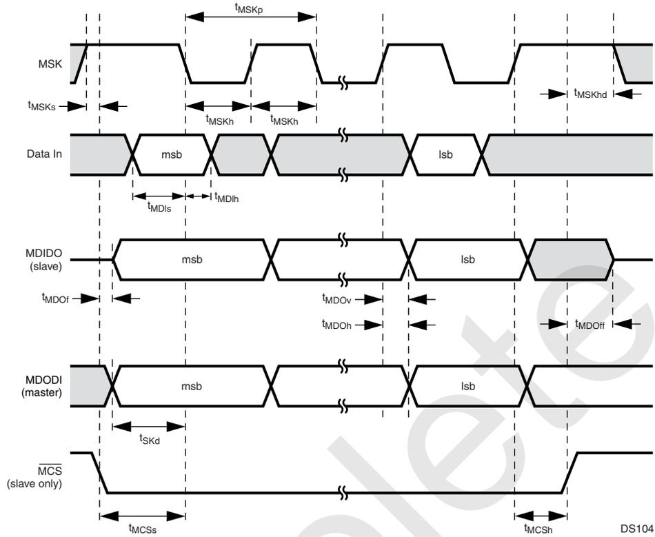
Figure 71. Microwire Transaction Timing, Alternate Mode, SCIDL = 1
