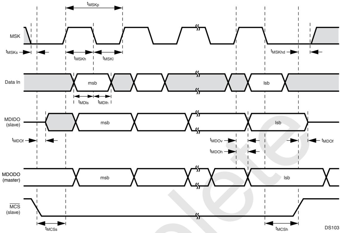
Figure 70. Microwire Transaction Timing, Alternate Mode, SCIDL = 0
