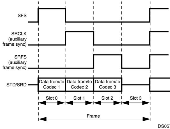
**Figure 21. Accessing Three Devices in Network Mode**
