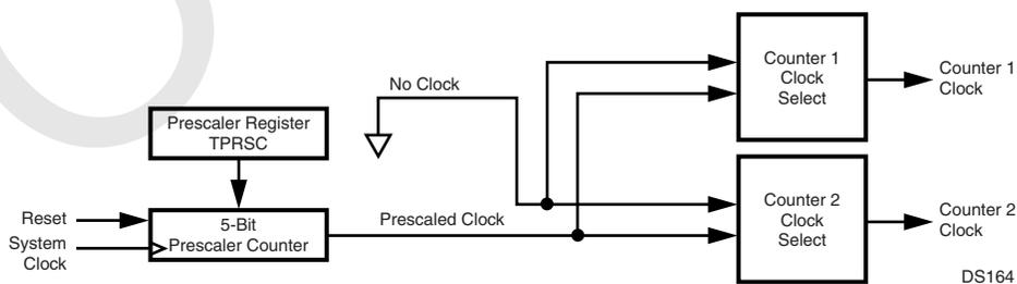
Figure 49. Multi-Function Timer Clock Source
