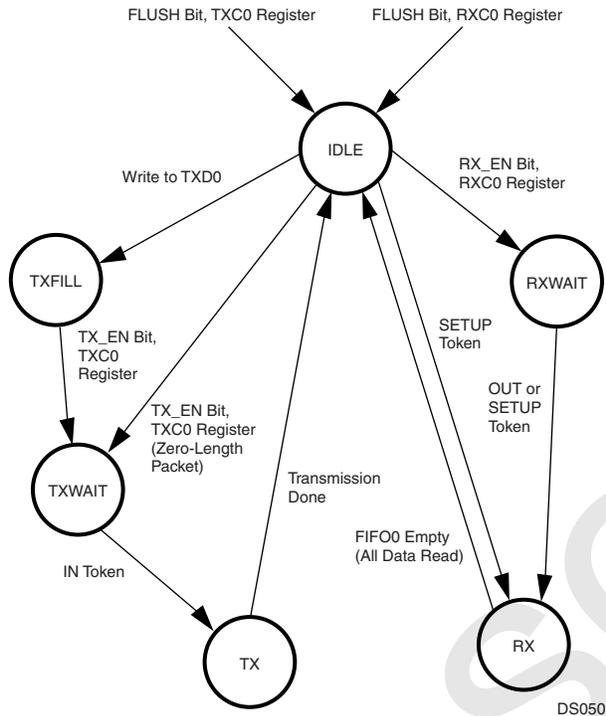
**Figure 13. Endpoint 0 Operation**
