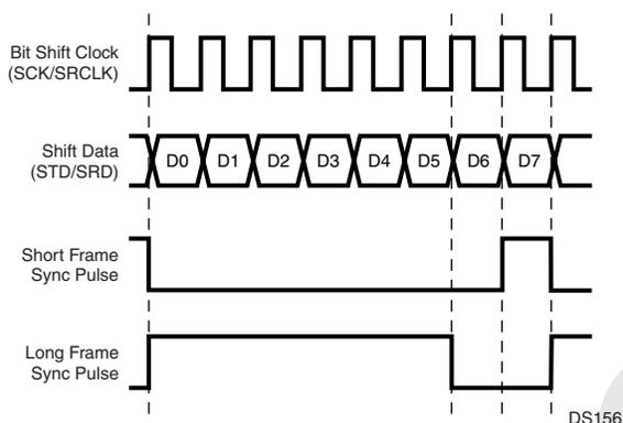
**Figure 23. Short and Long Frame Sync Pulses**
