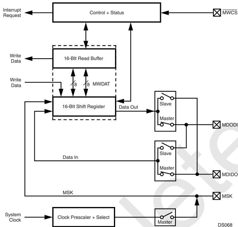
Figure 35. Microwire Block Diagram
