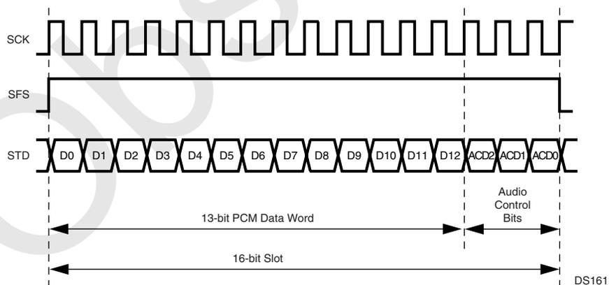
**Figure 24. Audio Slot with Audio Control Data**
