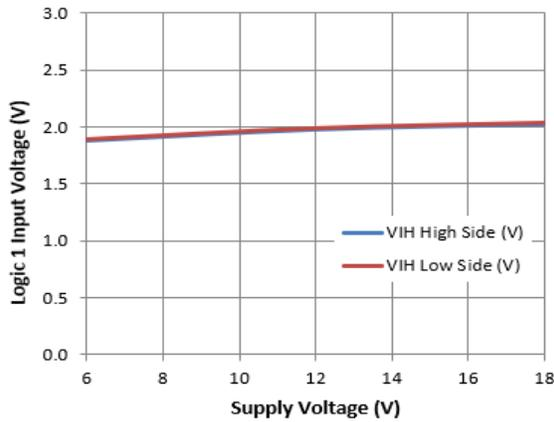
**Figure 20.** Logic 1 Input Voltage vs. Supply Voltage
