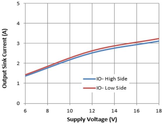
**Figure 18.** Output Sink Current vs. Supply Voltage
