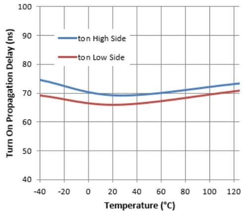
**Figure 5.** Turn-on Propagation Delay vs. Temperature
