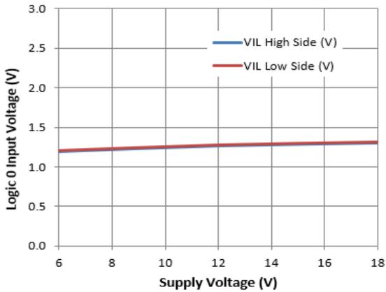
**Figure 22.** Logic 0 Input Voltage vs. Supply Voltage
