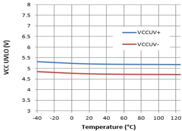
**Figure 24.** VCC UVLO vs. Temperature
