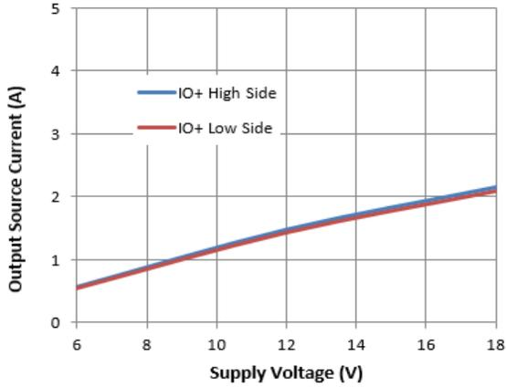
**Figure 16.** Output Source Current vs. Supply Voltage
