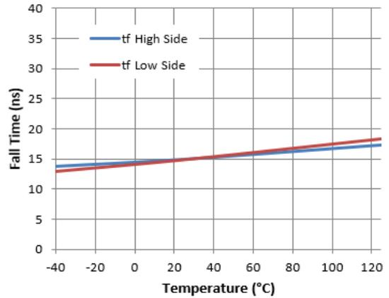
**Figure 11.** Fall Time vs. Temperature
