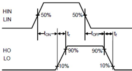
**Figure 1. Switching Time Waveform Definitions**
