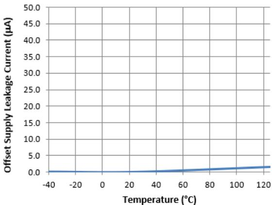
**Figure 26.** Offset Supply Leakage Current vs. Temperature
