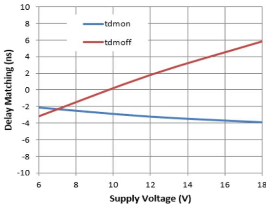
**Figure 14.** Delay Matching vs. Supply Voltage
