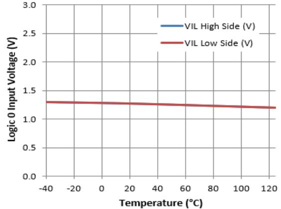
**Figure 23.** Logic 0 Input Voltage vs. Temperature
