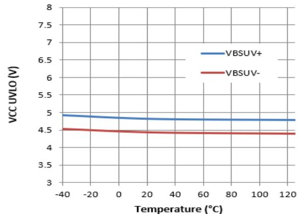
**Figure 25.** VBS UVLO vs. Temperature
