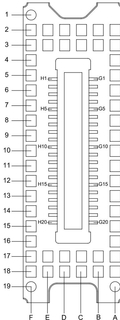
**Figure 5-1. FQJ Package. 40-Pin CLGA. Bottom View.**
