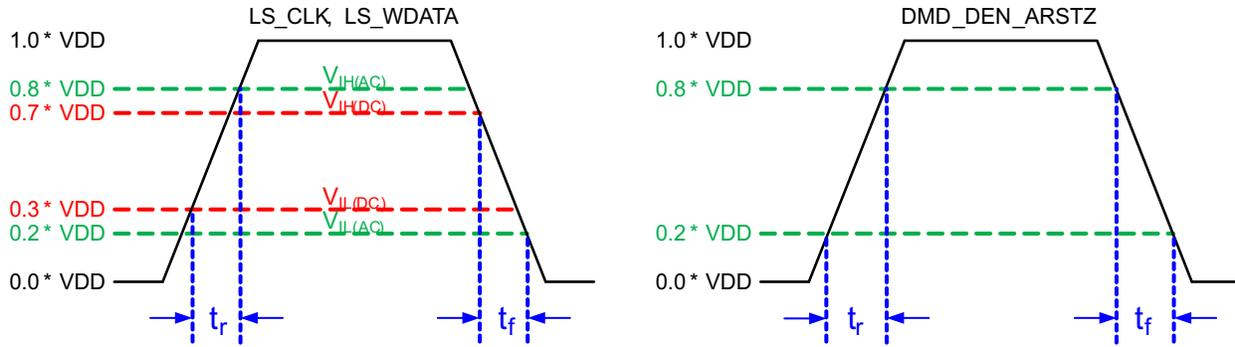
**Figure 6-3. LPSDR Input Rise and Fall Slew Rate**
