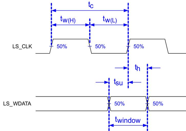
Low-speed interface is LPSDR and adheres to the [Electrical Characteristics](#) and AC/DC Operating Conditions table in JEDEC Standard No. 209B, *Low Power Double Data Rate (LPDDR) JESD209B*.
