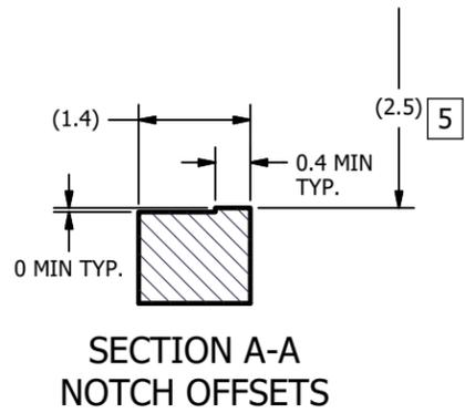
(PANASONIC AXT640124DD1, 40-CONTACT, 0.4 mm PITCH BOARD-TO-BOARD CONNECTOR HEADER) MATES WITH PANASONIC AXT540124DD1 OR EQUIVALENT CONNECTOR SOCKET
