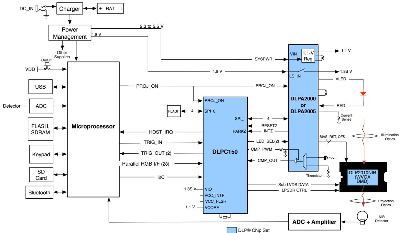
**Figure 8-1. Typical Application Diagram**
