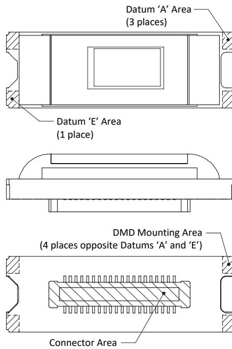
**Figure 6-14. System Interface Loads**
