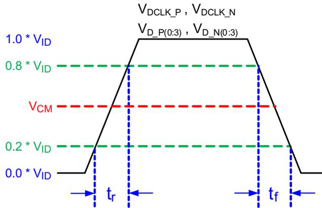
**Figure 6-4. SubLVDS Input Rise and Fall Slew Rate**
