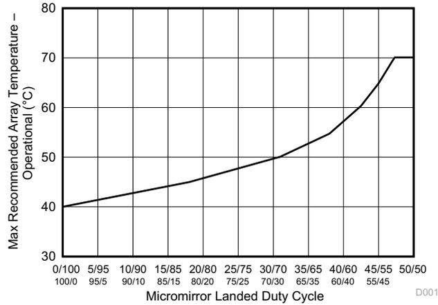
Figure 6-1. Maximum Recommended Array Temperature – Derating Curve
