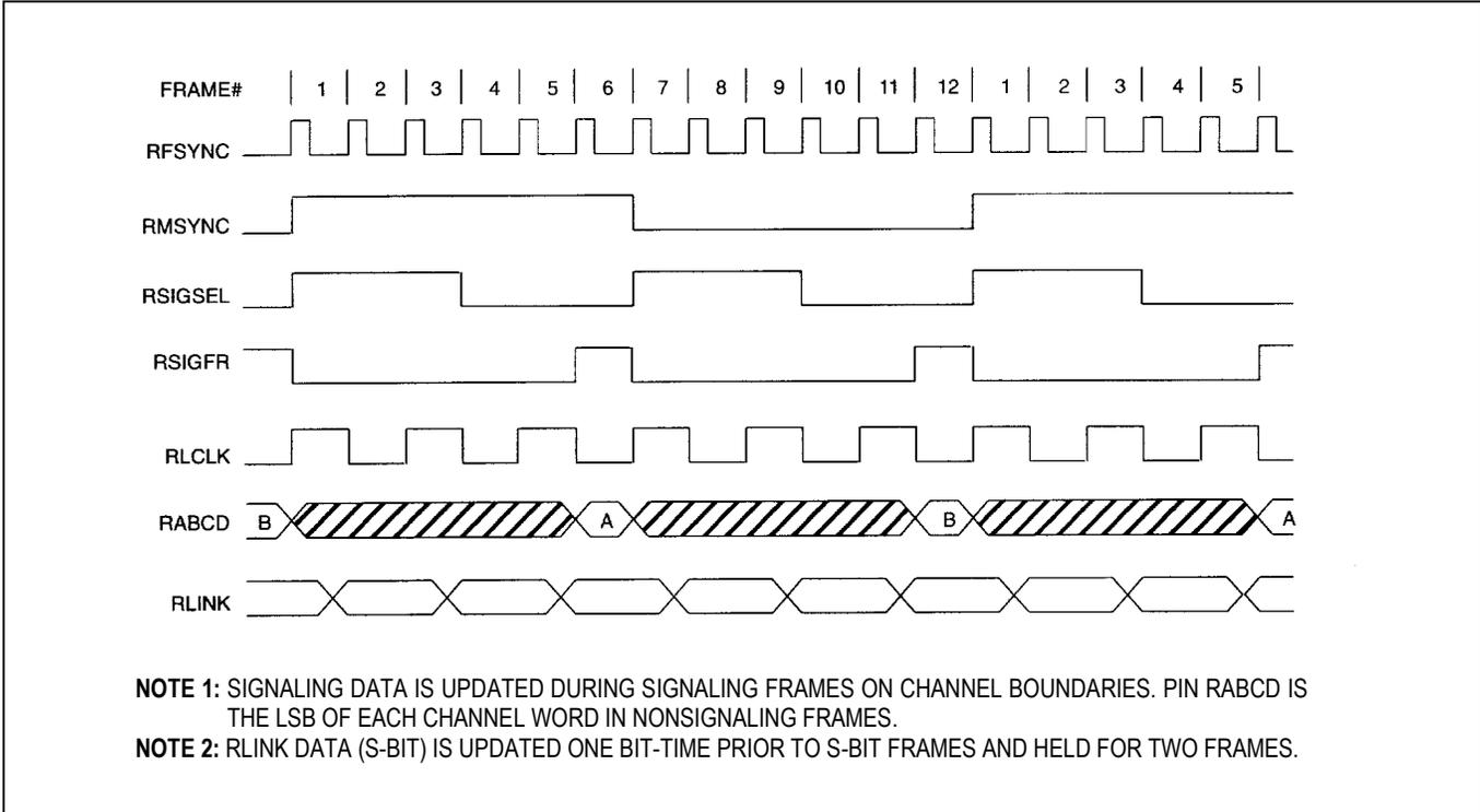
Figure 4. 193E Receive Multiframe Timing
