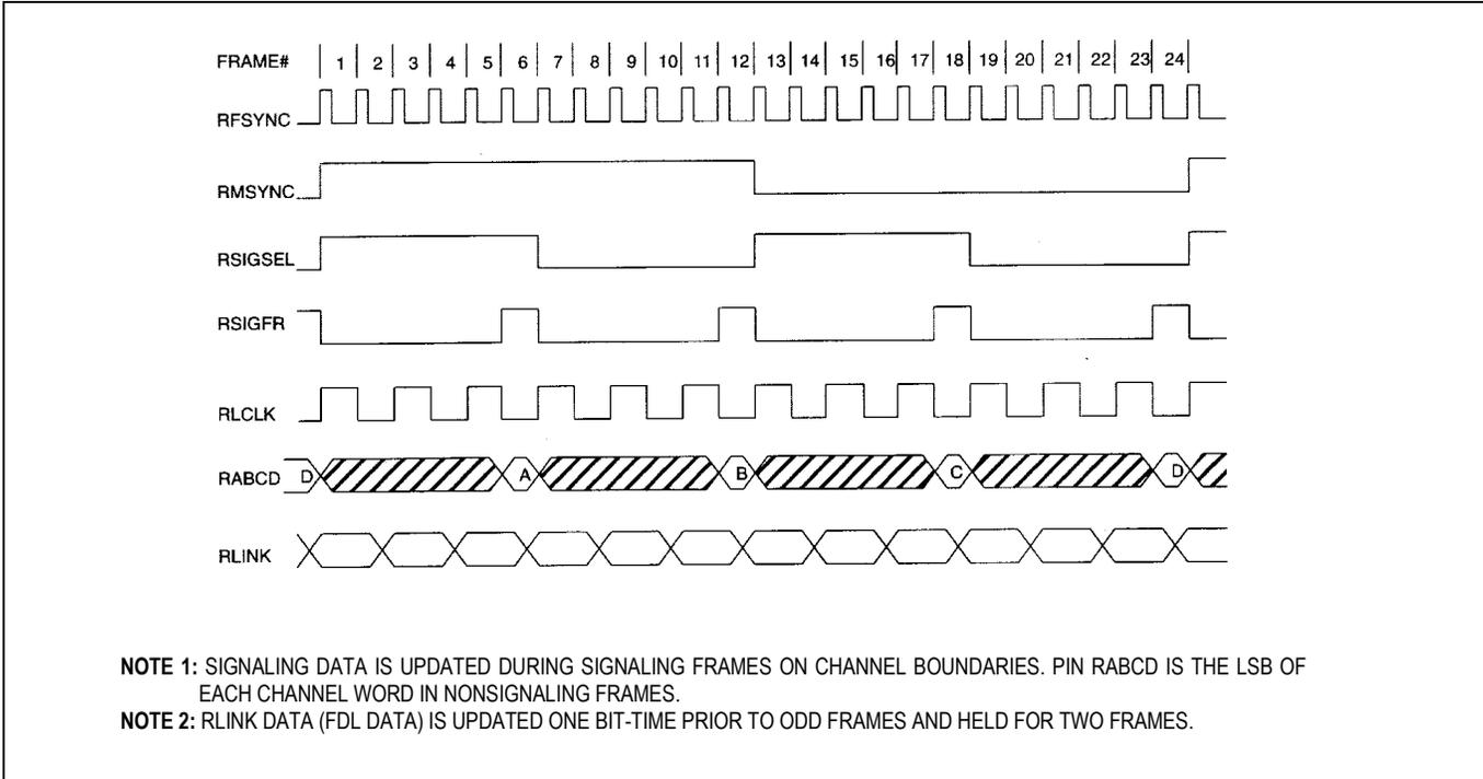
Figure 5. Receive Multiframed Boundary Timing
