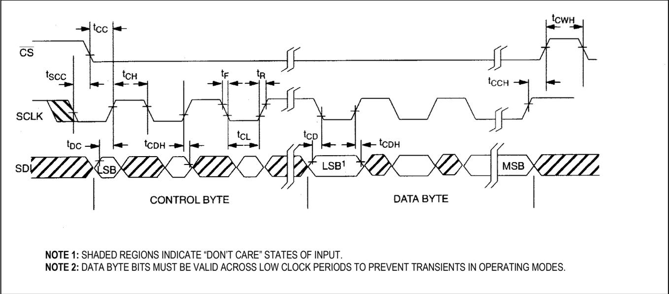
Figure 8. Serial Port Read AC Timing Diagram
