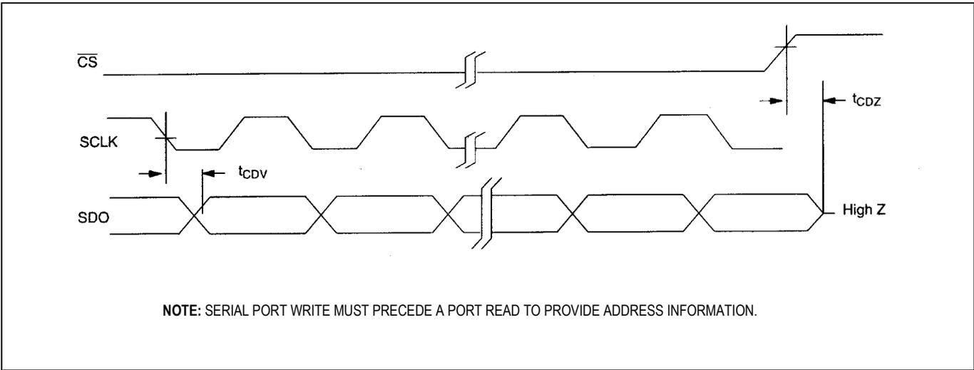
Figure 9. Receive AC Timing Diagram
