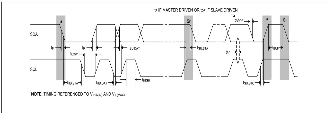
Figure 9. I<sup>2</sup>C Timing Diagram
