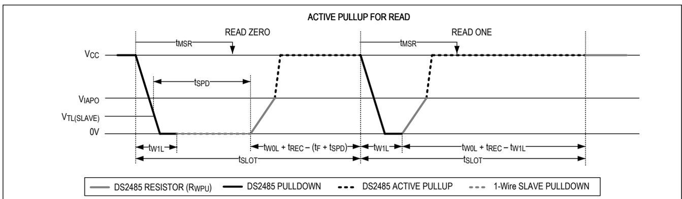
Figure 6. Active Pullup for 1-Wire Read Time Slot
