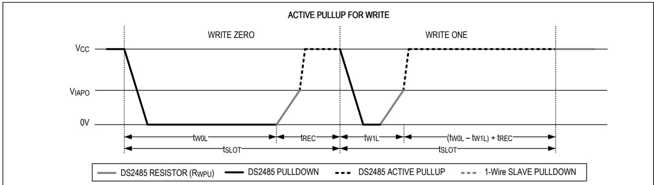
Figure 5. Active Pullup for 1-Wire Write Time Slot
