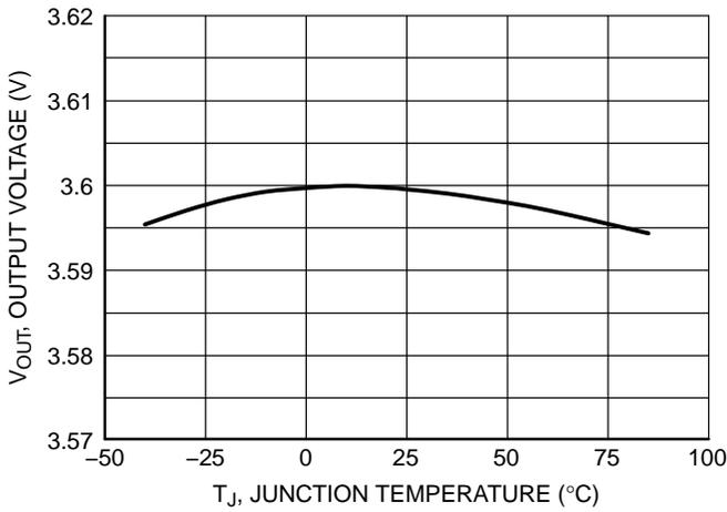
Figure 11. Output Voltage vs. Temperature, 3.6 V Version
