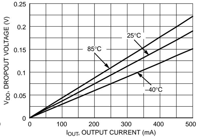
Figure 14. Dropout Voltage vs. Output Current, 3.6 V Version
