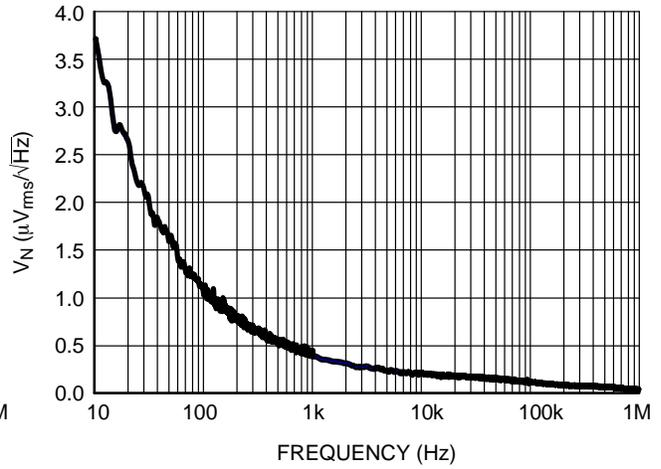
Figure 22. Output Noise vs. Frequency, 2.5 V Version
