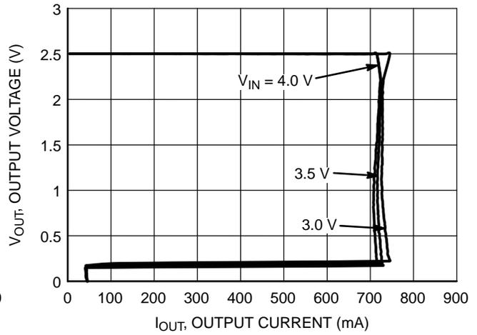
Figure 4. Output Voltage vs. Output Current 2.5 V Version
