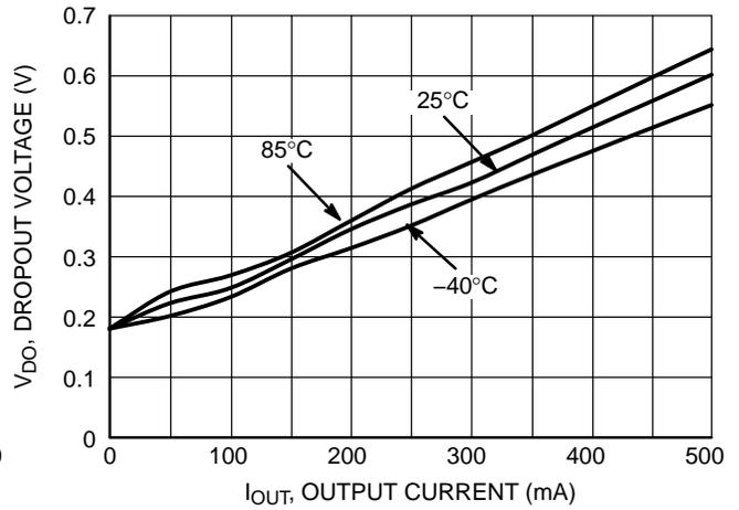
Figure 12. Dropout Voltage vs. Output Current, 0.7 V Version
