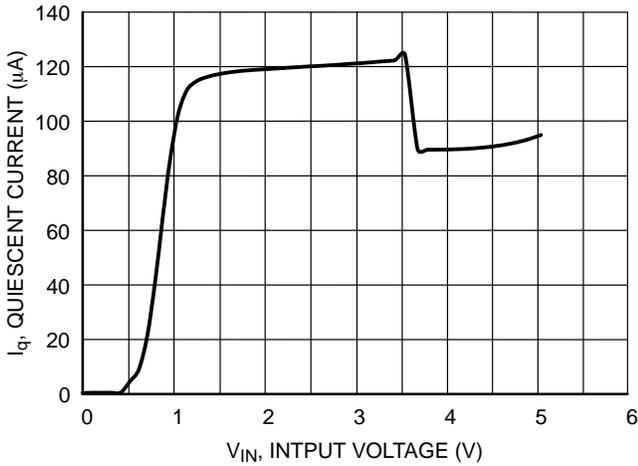
Figure 17. Quiescent Current vs. Input Voltage, 3.6 V Version
