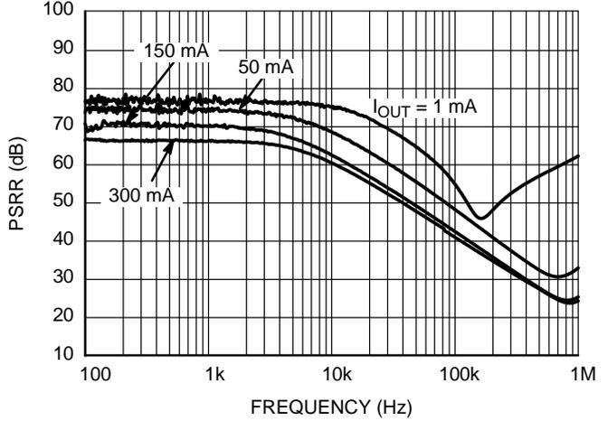
Figure 18. PSRR vs. Frequency, 0.7 V Version
