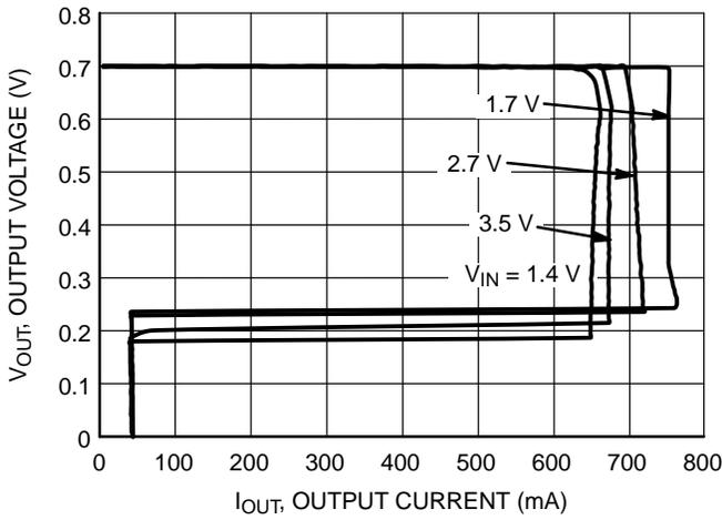
Figure 3. Output Voltage vs. Output Current 0.7 V Version
