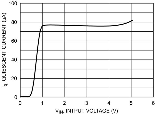
Figure 15. Quiescent Current vs. Input Voltage, 0.7 V Version
