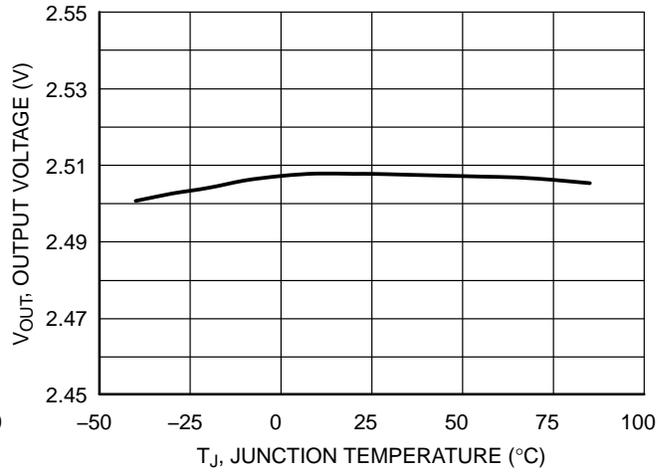
Figure 10. Output Voltage vs. Temperature, 2.5 V Version
