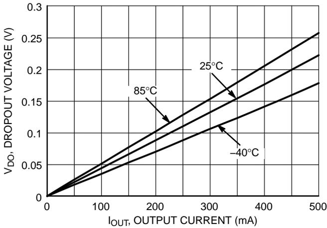
Figure 13. Dropout Voltage vs. Output Current, 2.5 V Version
