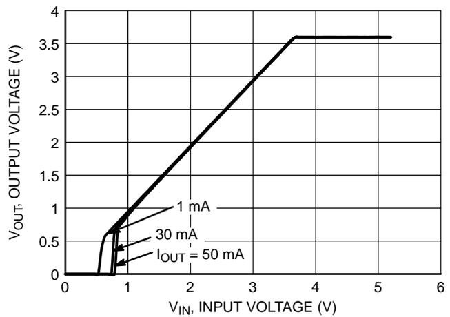
Figure 8. Output Voltage vs. Input Voltage 3.6 V Version
