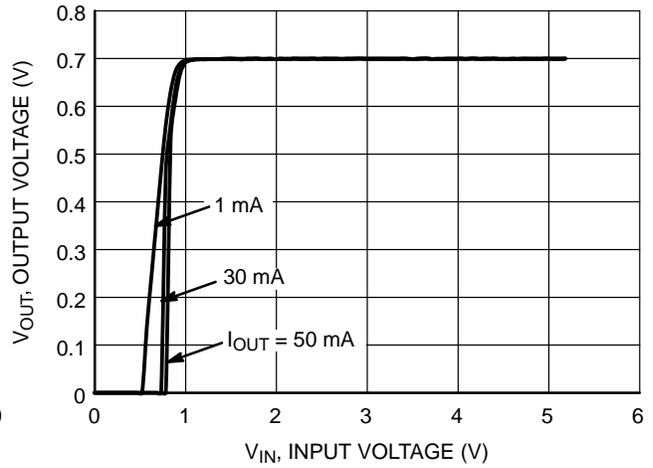
Figure 6. Output Voltage vs. Input Voltage 0.7 V Version
