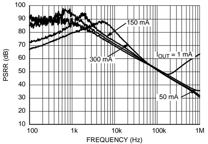
Figure 20. PSRR vs. Frequency, 3.6 V Version
