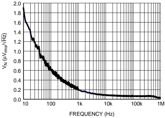
Figure 21. Output Noise vs. Frequency, 0.7 V Version
