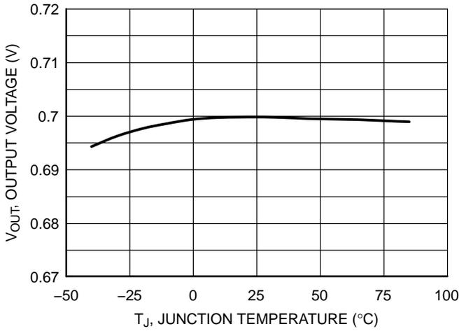
Figure 9. Output Voltage vs. Temperature, 0.7 V Version
