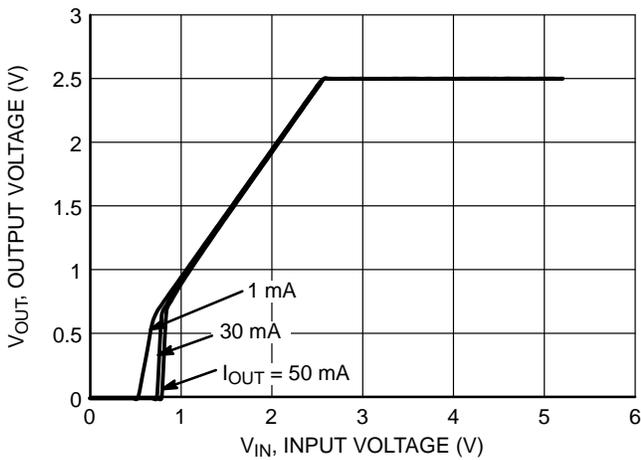
Figure 7. Output Voltage vs. Input Voltage 2.5 V Version
