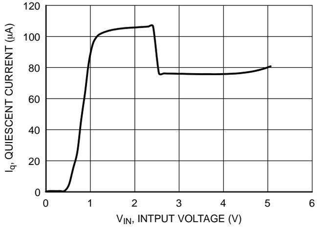
Figure 16. Quiescent Current vs. Input Voltage, 2.5 V Version
