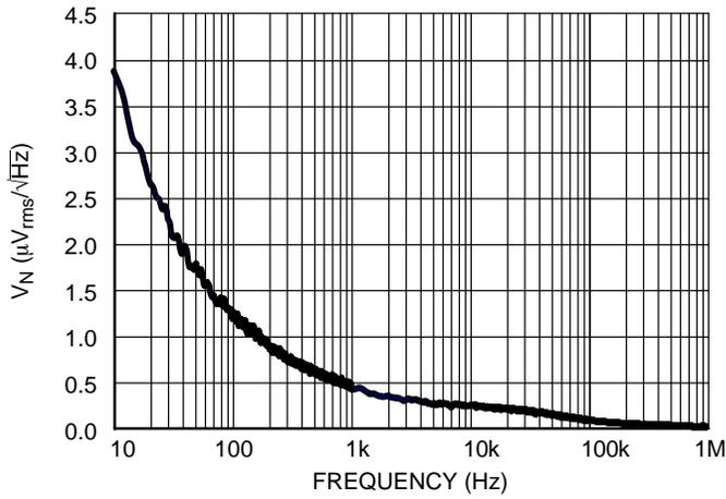
Figure 23. Output Noise vs. Frequency, 3.6 V Version
