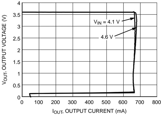
Figure 5. Output Voltage vs. Output Current 3.6 V Version
