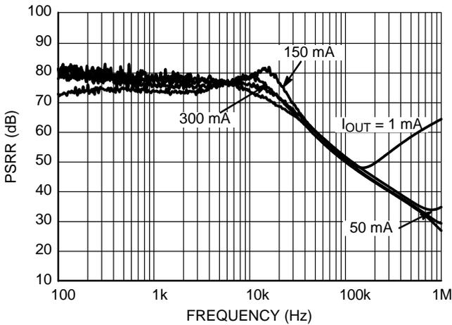
Figure 19. PSRR vs. Frequency, 2.5 V Version
