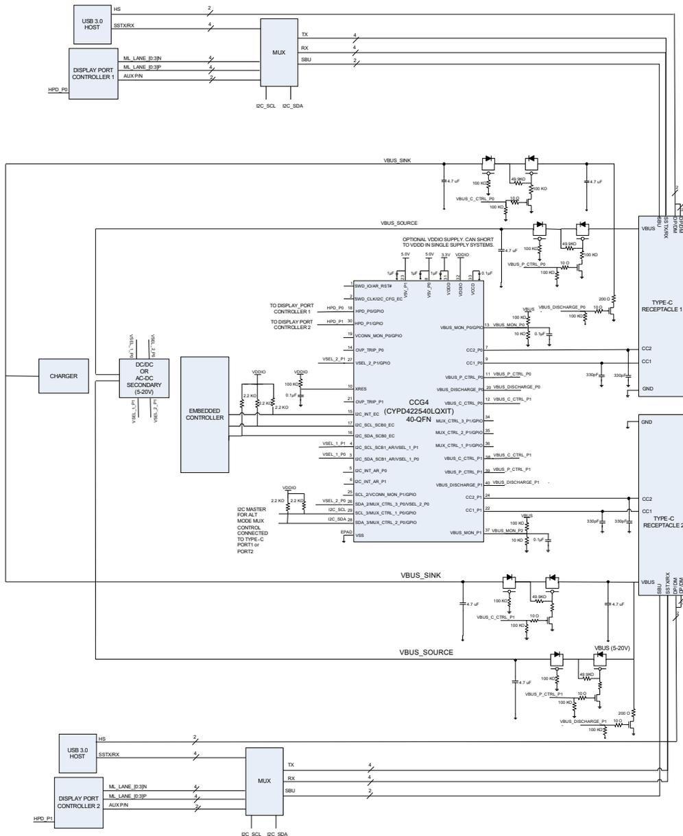
**Figure 9. CCG4 in a Single Port Notebook Application using CYPD4125-40LQXIT**
