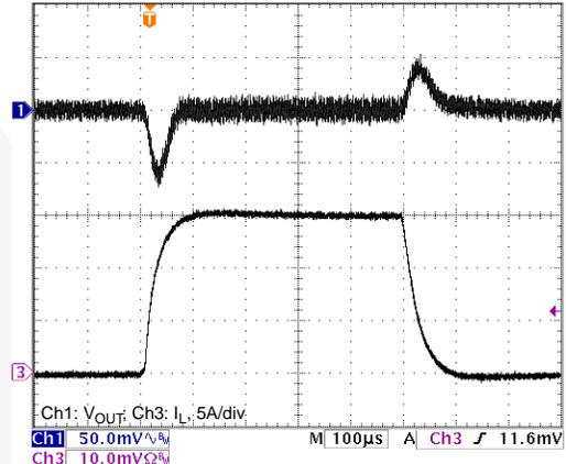
Figure 6. PWM Load Transient (0 to 15A)
