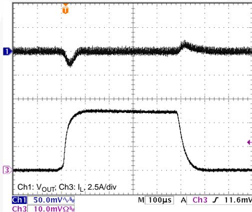
Figure 4. PWM Load Transient (0 to 5A)
