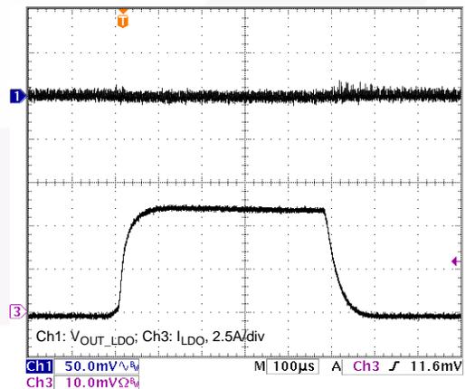
Figure 8. LDO Load Transient (0 to 5A)
