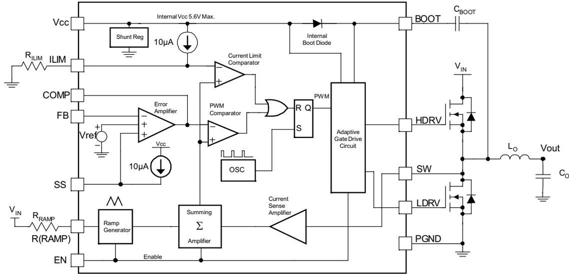
Figure 21. Block Diagram
