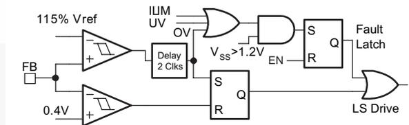
Figure 22. Over-Voltage Protection
