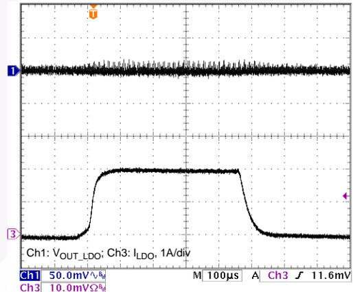
Figure 7. LDO Load Transient (0 to 2A)
