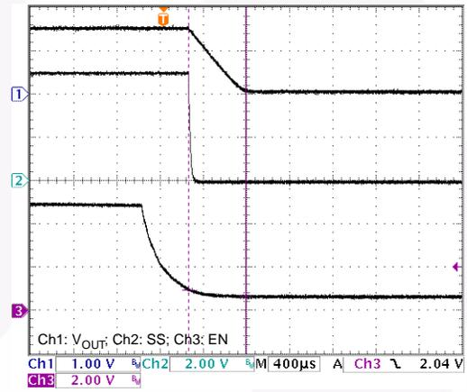
Figure 13. Enable Off ( $I_{PWM} = 5A$ )
