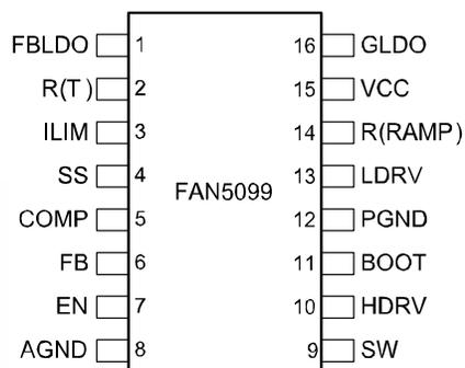
Figure 2. Pin Assignment
