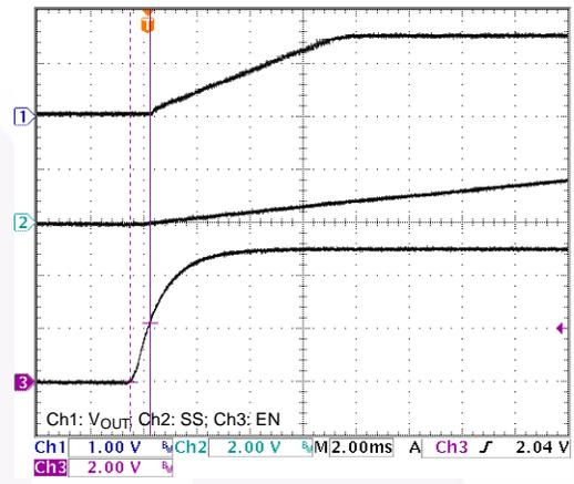
Figure 12. Enable On ( $I_{PWM} = 5A$ )
