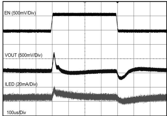
Figure 19. Line Transient Response for 5 LEDs
