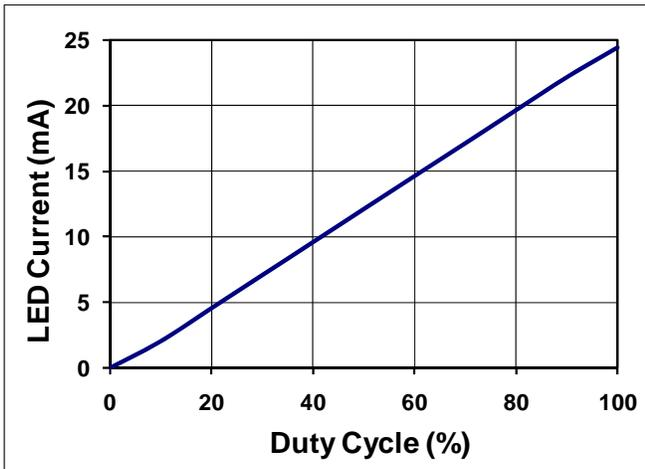
Figure 18. LED Current vs. Duty Cycle,  $f_{PWM} = 20kHz$
