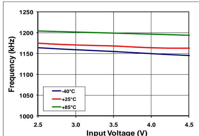
Figure 13. Frequency vs. Input Voltage vs. Temperature
