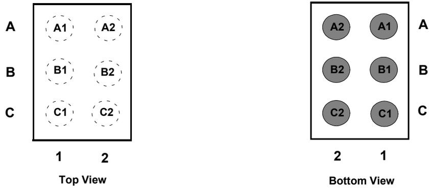
Figure 3. Pin Assignments
