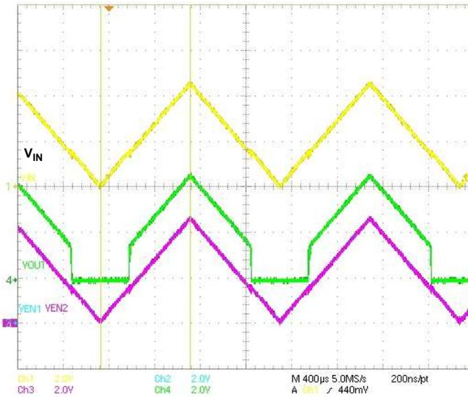
Figure 22.  $V_{IN}$  Ramp Up and Down ( $EN1 = EN2 = V_{IN} = 0$  to 4.8 V (6100 V/sec),  $C_{OUT} = 50$  pF,  $R_L = 500 \Omega$ , timescale = 400  $\mu$ s/div)
