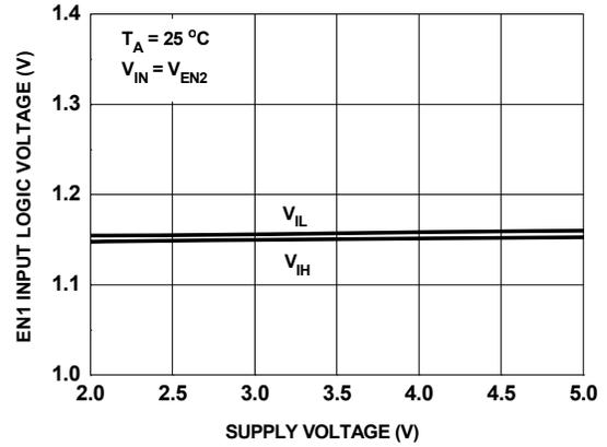
Figure 12. EN1 Logic Voltage vs Supply Voltage ( $V_{IN}$ )
