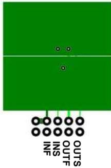
a. 115 °C/W when mounted on a 1 in<sup>2</sup> pad of 2 oz copper.
