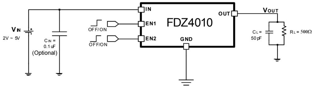
Figure 23. Typical Application Circuit
