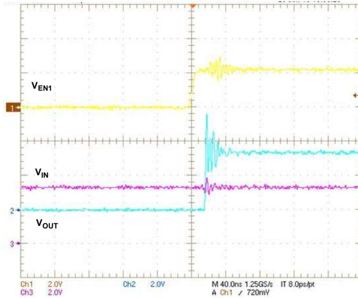
Figure 19. Turn-On Time ( $V_{IN} = 3.3\text{ V}$ ,  $V_{EN2} = 2.3\text{ V}$ ,  $V_{EN1} = 0$  to  $2.3\text{ V}$ ,  $C_{OUT} = 50\text{ pF}$ ,  $R_L = 500\ \Omega$ , timescale =  $40\ \mu\text{s}/\text{div}$ )
