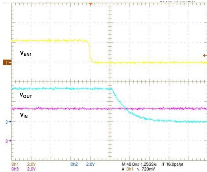
Figure 20. Turn-Off Time ( $V_{IN} = 3.3\text{ V}$ ,  $V_{EN2} = 2.3\text{ V}$ ,  $V_{EN1} = 2.3$  to  $0\text{ V}$ ,  $C_{OUT} = 50\text{ pF}$ ,  $R_L = 500\ \Omega$ , timescale =  $40\ \mu\text{s}/\text{div}$ )
