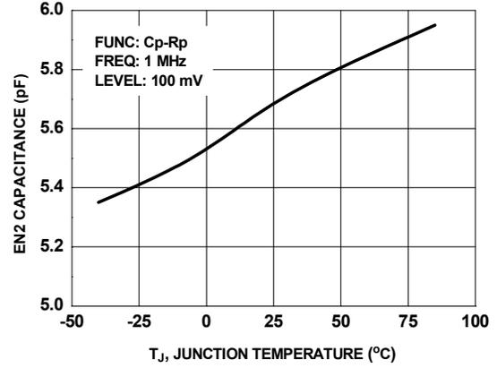
Figure 18. EN2 Capacitance vs Temperature
