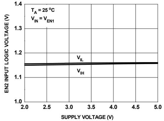
Figure 14. EN2 Logic Voltage vs Supply Voltage ( $V_{IN}$ )
