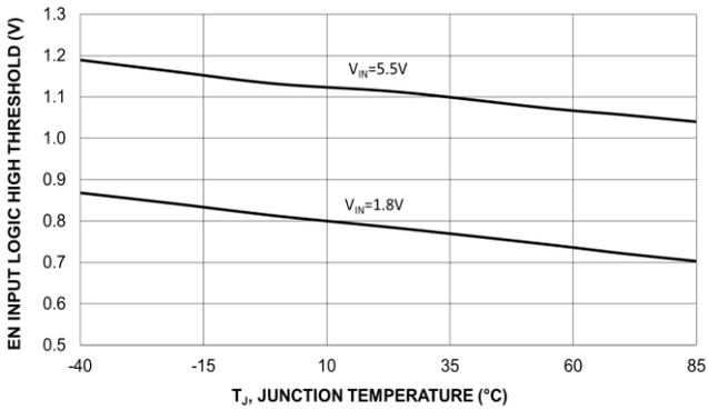
Figure 10. EN Input Logic High Threshold Vs. Temperature
