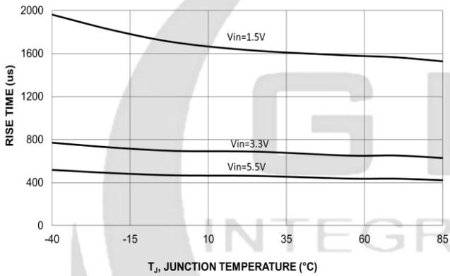
Figure 22.  $V_{OUT}$  Rise Time vs. Temperature
