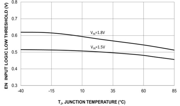
Figure 11. EN Input Logic Low Threshold Vs. Temperature
