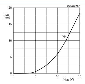
Fig. 6. Typical supply current as a function of supply
