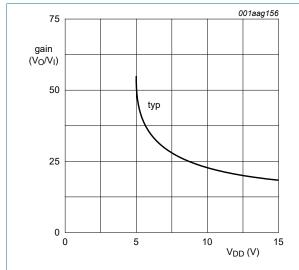
Fig. 5. Typical voltage gain as a function of supply voltage
