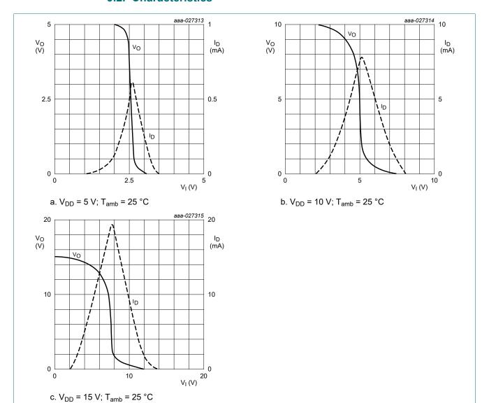
Fig. 4. Typical drain current  $I_D$  and output voltage  $V_O$  as functions of input voltage
