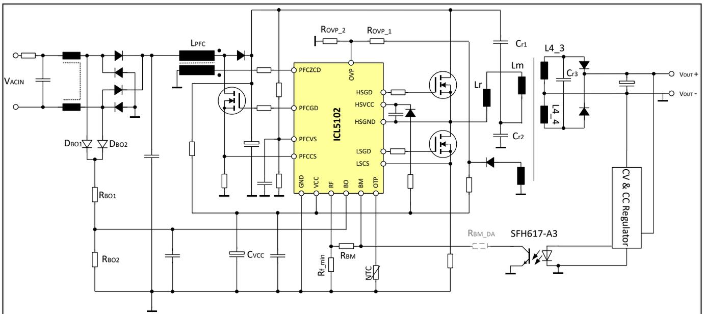
**Figure 1 ICL5102 Typical Application with PFC+LLC Topology**
