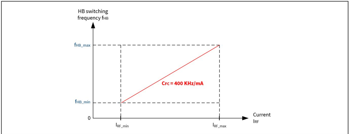
**Figure 13** CCO of ICL5102 in Normal Operation
