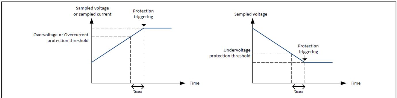
**Figure 11** Excess of threshold due to Blanking Time
