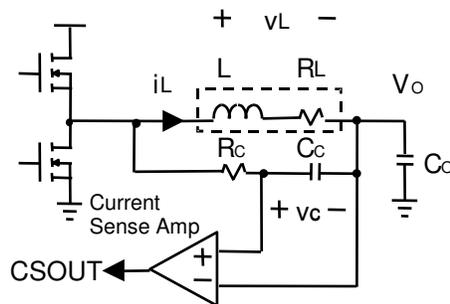
Figure 8: Inductor Current Sensing and Current Sense Amplifier
