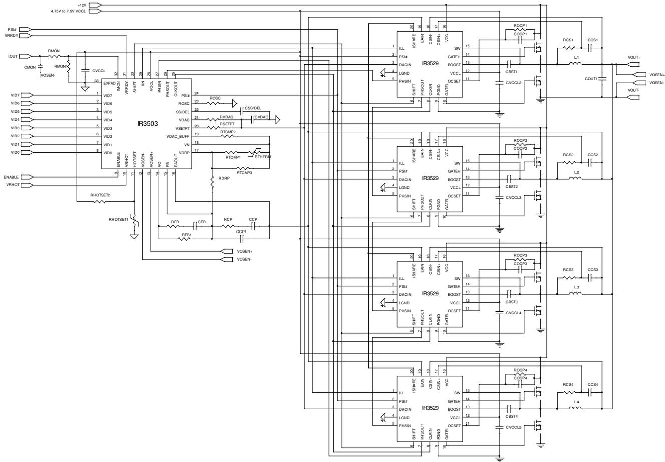
**Note:** Pin 33 of IR3503 is the exposed pad located under the IC. It is connected to IC ground
