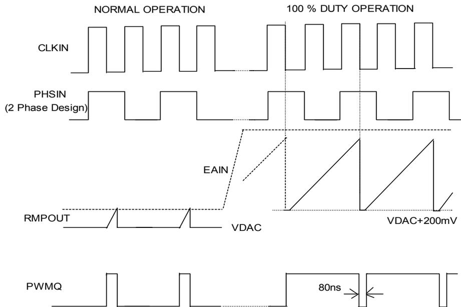
Figure 7: PWM Operation during normal and 100 % duty mode.
