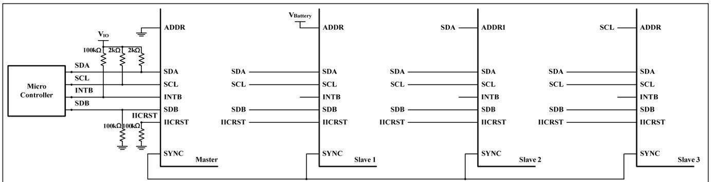
Figure 3 Typical Application Circuit (Four Parts Synchronization-Work)
