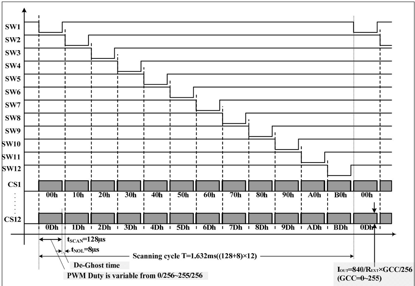
Figure 12 Scanning Timing
