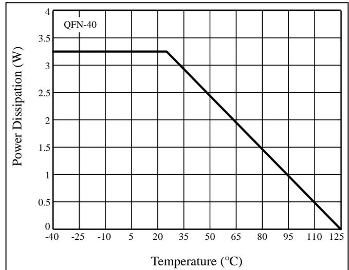
**Figure 17** Dissipation Curve
