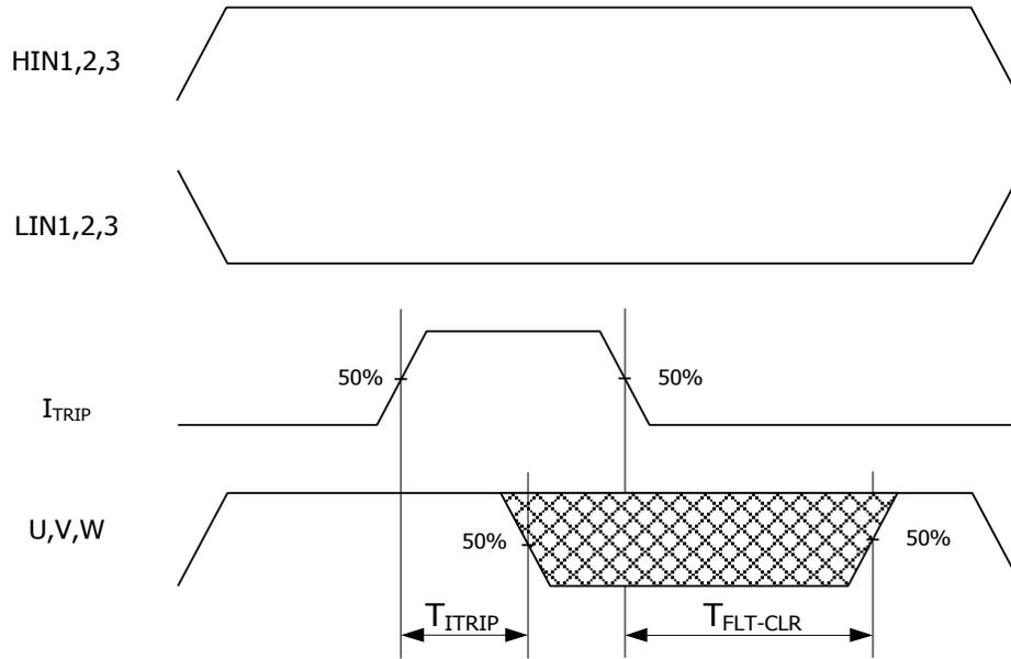
**Figure 3: I<sub>TRIP</sub> Timing Waveform**
