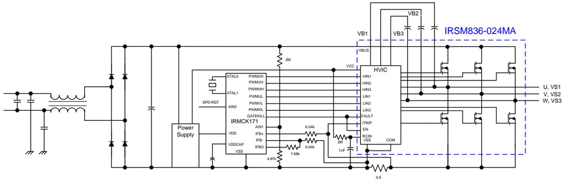
1. Electrolytic bus capacitors should be mounted as close to the module bus terminals as possible to reduce ringing and EMI problems. Additional high frequency ceramic capacitor mounted close to the module pins will further improve performance.
