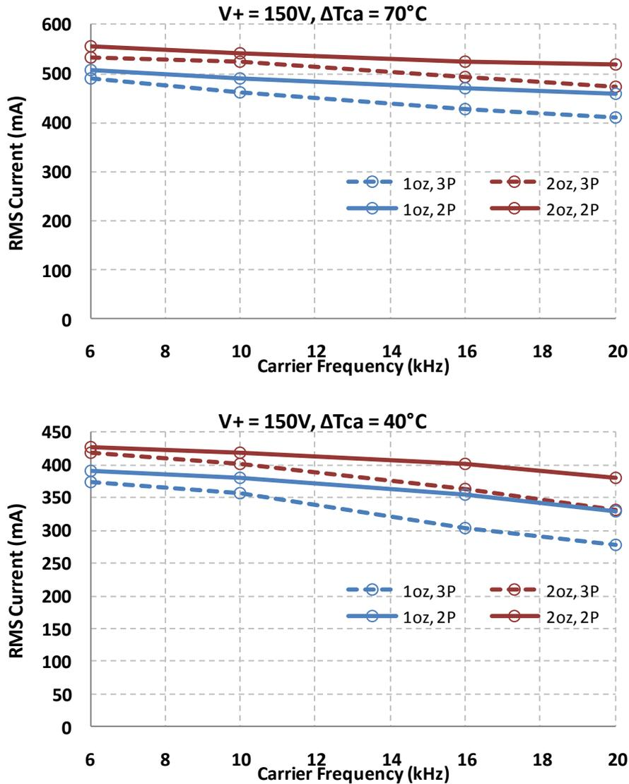
Figure 6: Maximum Sinusoidal Phase Current vs. PWM Switching Frequency
