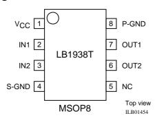
S-GND: GND for the control system P-GND: GND for the power system
