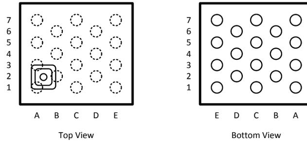
**Figure 1. 18-Bump Thin DSBGA Package, Large Bump Package Number YZR0018**
