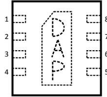
**Figure 2. 8-Lead Thin WSON Package
