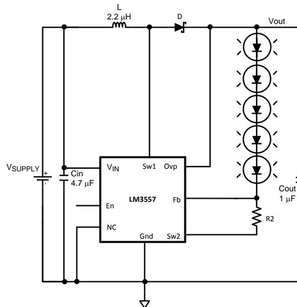
**Figure 1. Backlight Configuration**
